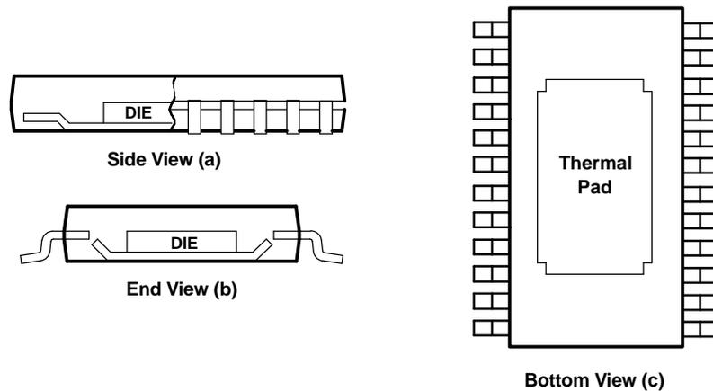
**Figure 41. Views of Thermally Enhanced PWP Package**
