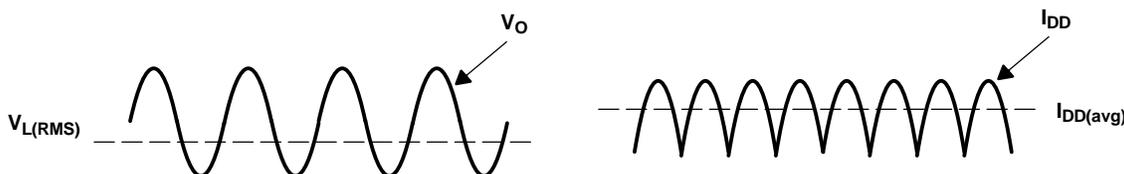
Figure 46. Voltage and Current Waveforms for BTL Amplifiers
