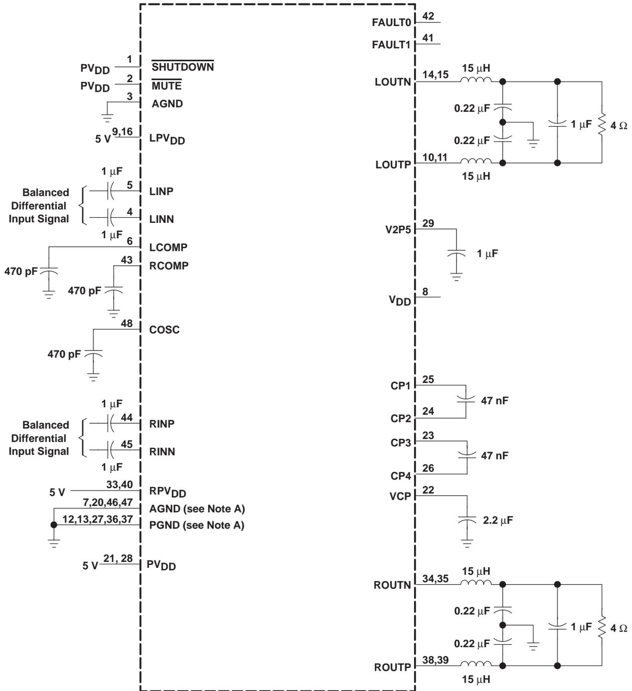
Figure 1. 5-V, 4-Ω Test Circuit, Class-D Amplifier
