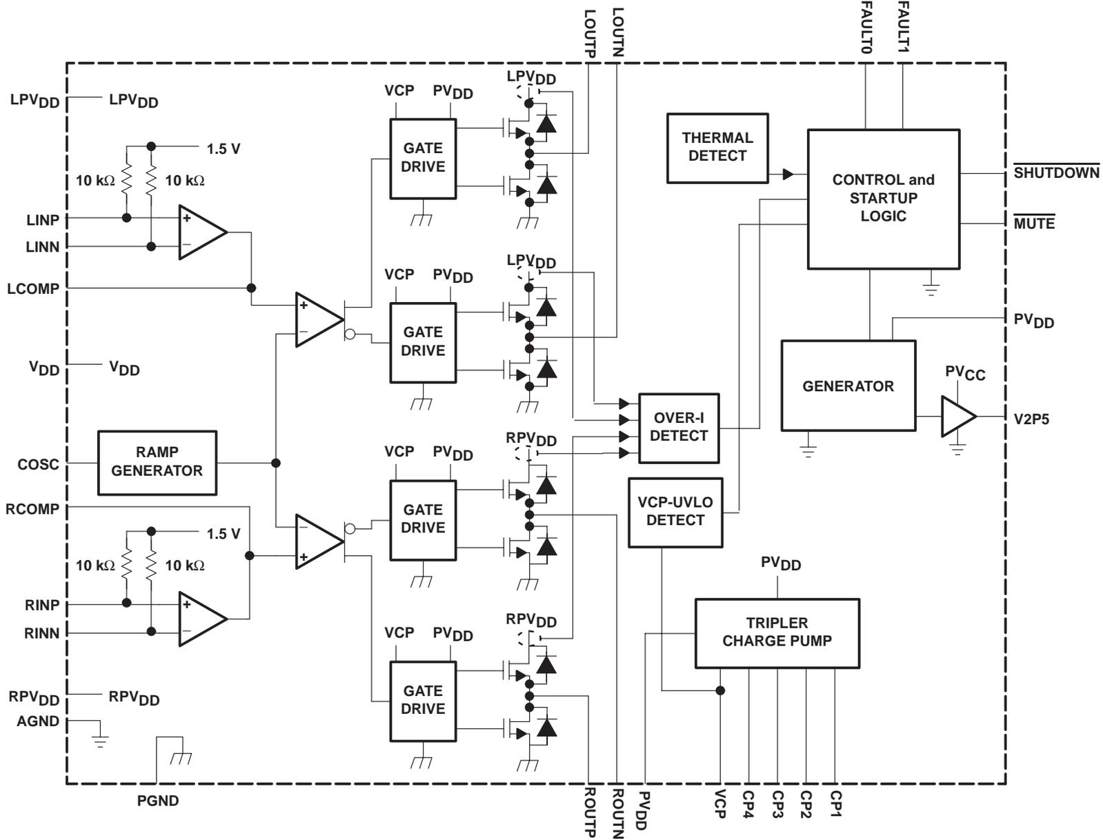
NOTE A: LPVDD, RPVDD, VDD, and PVDD are externally connected. AGND and PGND are externally connected.
