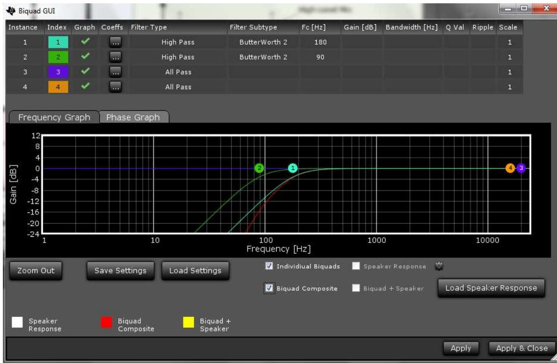
Figure 54. HF4 DBE EQ High-Level Tuning Window
