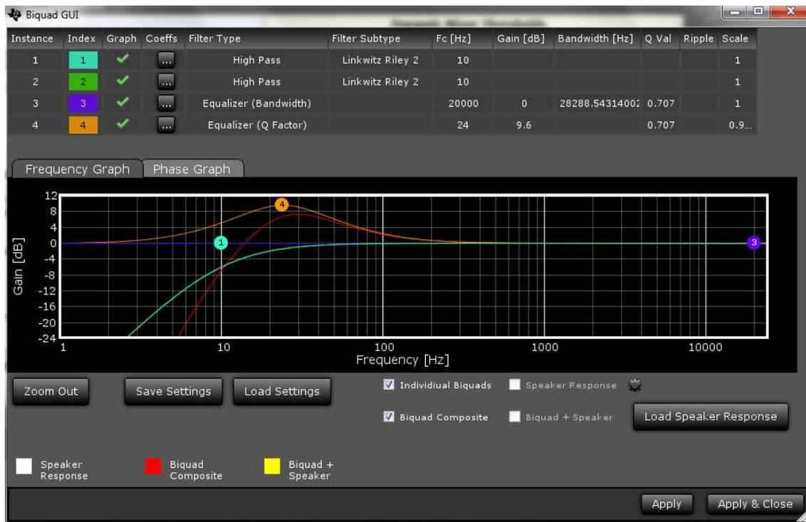
Figure 53. HF4 DBE EQ Low-Level Tuning Window
