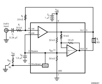
FIGURE 1. Typical Audio Amplifier Application Circuit
