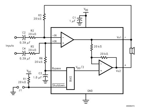
FIGURE 2. Differential Amplifier Configuration for LM4900
