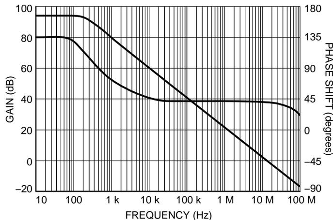
Figure 22. Gain and Phase Shift vs. Frequency
