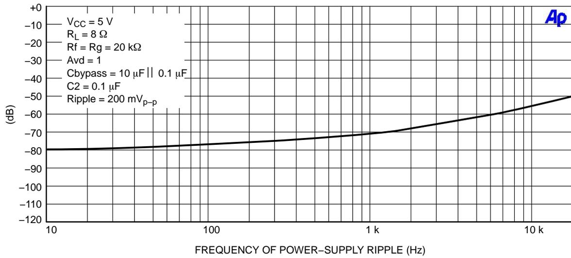
Figure 23. Power-Supply Rejection
