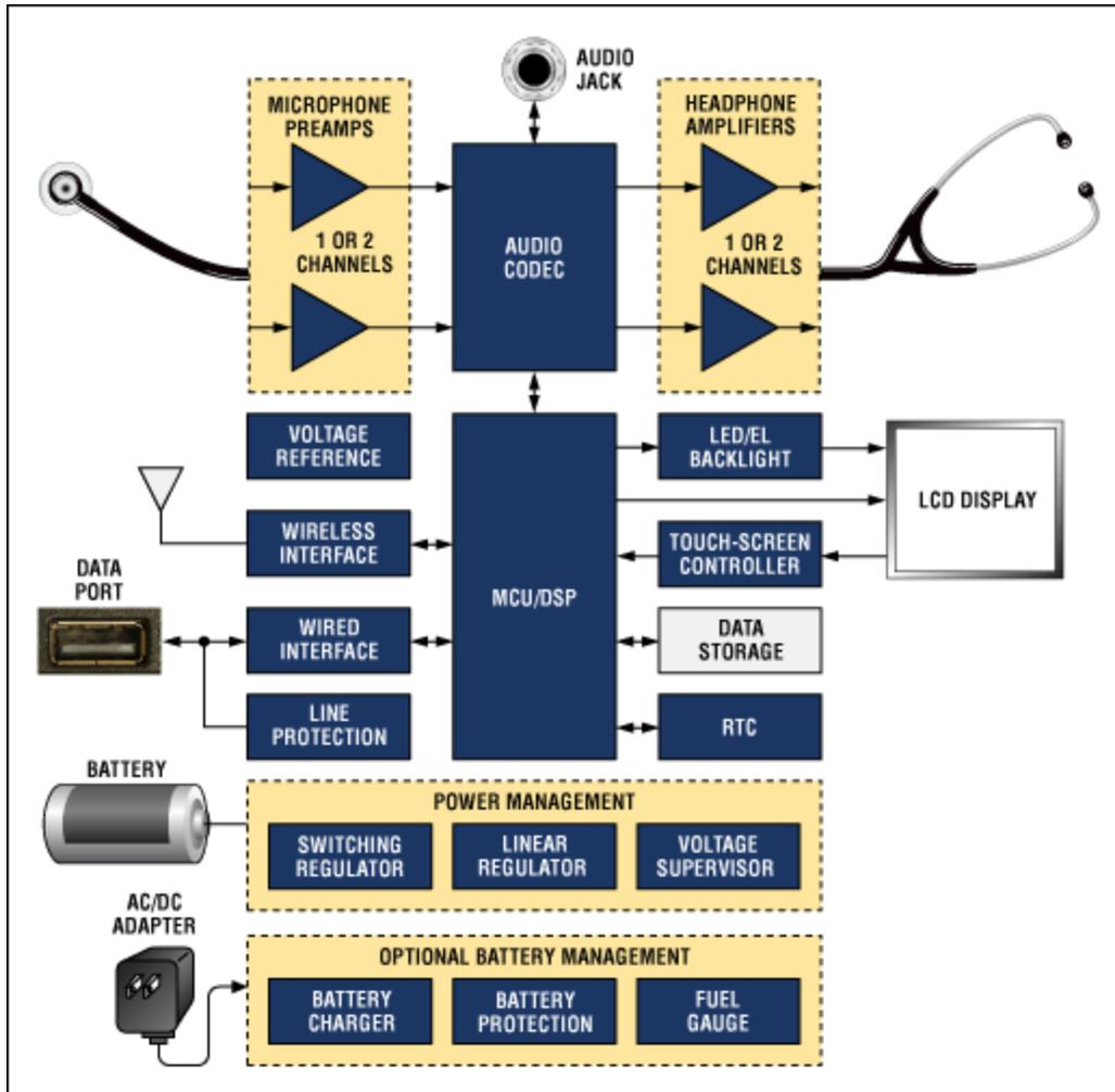
Functional block diagram of a digital stethoscope. For a list of Maxim's recommended digital-stethoscope solutions, please go to: [www.maximintegrated.com/stethoscope](http://www.maximintegrated.com/stethoscope).
