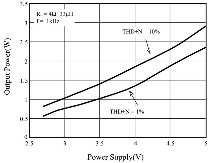
**Figure 10** Output Power vs. Supply Voltage
