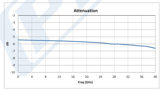
Click the following link (or enter part number in "SEARCH" on website) to obtain additional part information including price, inventory and certifications: 6 dB Fixed Attenuator, 2.92mm Male to 2.92mm Female Passivated Stainless Steel Body Rated to 2 Watts Up to 40 GHz PE7395-6
