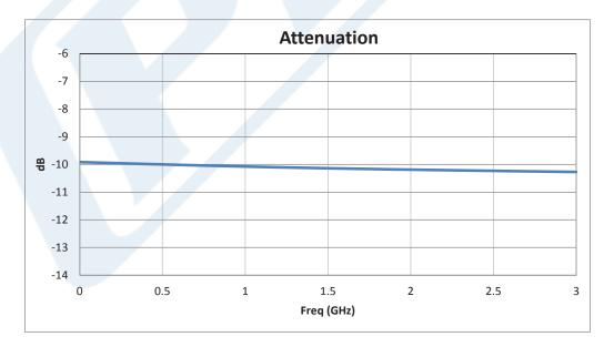
Click the following link (or enter part number in "SEARCH" on website) to obtain additional part information including price, inventory and certifications: 10 dB Fixed Attenuator, N Male to N Female Unidirectional Black Anodized Aluminum Heatsink Body Rated to 50 Watts Up to 3 GHz PE7388-10
