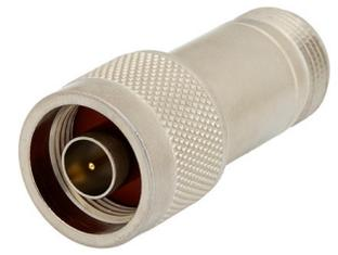
20 dB Fixed Attenuator, 75 Ohm N Male to 75 Ohm N Female Brass Nickel Body Rated to 2 Watts Up to 4 GHz
