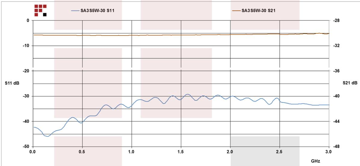
30 dB Fixed Attenuator SMA Male To SMA Female Up To 3 GHz Rated To 5 Watts With Aluminum Body from Fairview Microwave is in-stock and available to ship same-day. All of our RF/microwave products are available off-the-shelf from our ISO 9001:2008 certified facilities in Allen, Texas. Fairview Microwave is RF on-demand.
