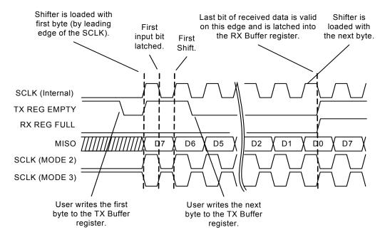
Figure 18-10. Typical SPIS Timing in Modes 2 and 3
