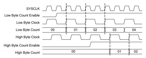
Figure 11-19. 6-Bit RLO Timer Operation
