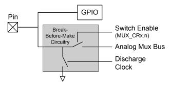
For each pin, the mux capability exists in parallel with the normal GPIO cell, shown in Figure 12-2. Normally, the associated GPIO pin is put into a high impedance state for these applications, although there are cases where the GPIO cell is configured by the user to briefly drive pin initialization states as described ahead.
