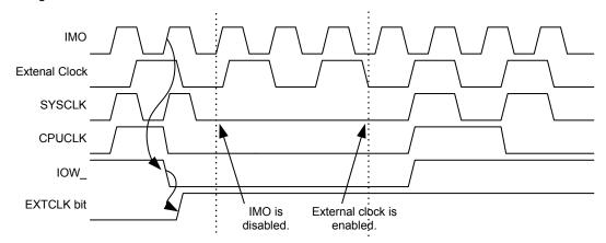
Figure 14-3. Switch from IMO to External Clock with the CPU Running with a CPU Clock Divider of One
