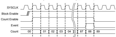
Figure 11-16. Pulse Width Frequency Timing (Mode = 01/10)
