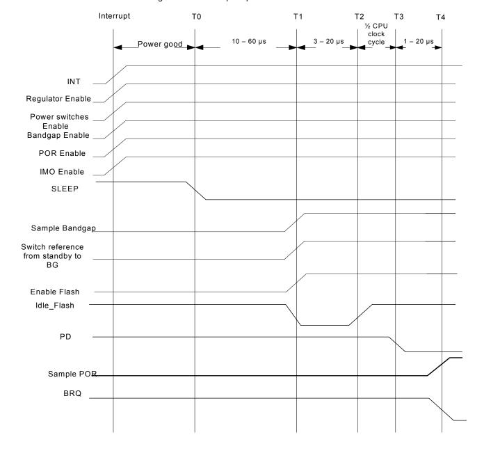
Figure 10-2. Wakeup Sequence for the Device 123
