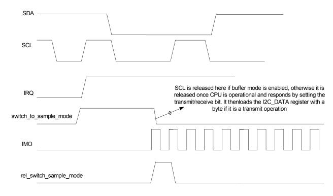
Figure 15-13. Direct Clocking to Sample Mode Timing
