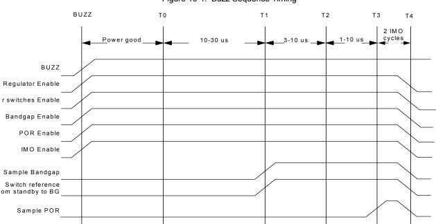
Figure 10-4. Buzz Sequence Timing
