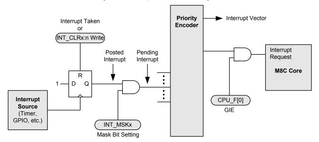
Figure 5-1. Interrupt Controller Block Diagram
