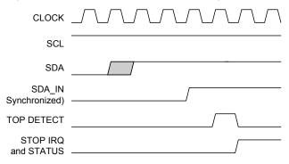
Figure 15-10 illustrates the timing for bus error interrupts. Bus Error status (and interrupt) occurs one cycle after the internal Start or Stop detect (two cycles after the filtered and synchronized SDA input transition).
