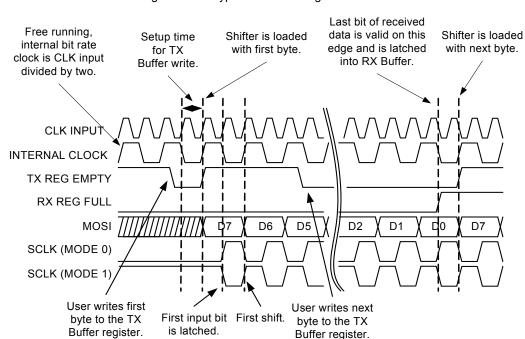
Figure 18-5. Typical SPIM Timing in Mode 0 and 1
