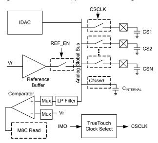
The reference bus is connected to the analog global line to initialize it to the Vr voltage (see Figure 11-7). After that, the reference buffer is disconnected and not used. The sense capacitance pin is now alternately grounded (see Figure 11-8) and connected to the analog global (see Figure 11-9). With the IDAC's current driving onto this net, the global net alternately charges and discharges a small amount.
