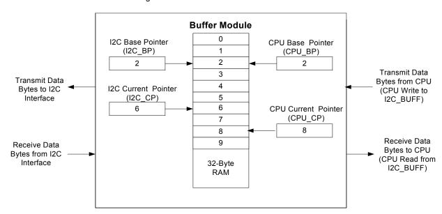
Figure 15-5. Address Pointer in EZI2C Mode
