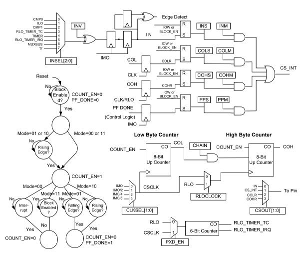
Figure 11-13. TrueTouch Counter Block Diagram
