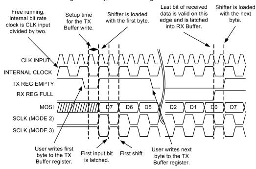
Figure 18-6. Typical SPIM Timing in Mode 2 and 3
