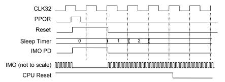
**XRES**: Reset while XRES is high (IMO off), then 7(+) cycles (IMO on), and then the CPU reset is released.
