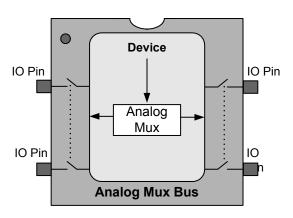
ber of pins can be enabled at the same time. At reset, all of these mux connections are open (disconnected).
