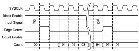
Figure 11-17. Continuous Timing (Mode = 11)
