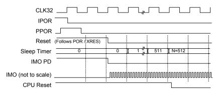
**PPOR** (with no IPOR): Reset while PPOR is high and to the end of the next 32K cycle (IMO off); 1 cycle IMO on before the CPU reset is released. Note that at the 3V level, PPOR tends to be brief because the reset clears the POR range register (VLT\_CR) back to the default 2.4V setting.
