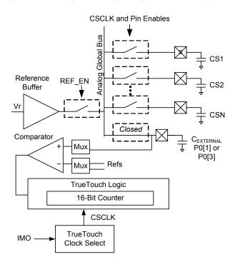
The initialization phase for negative CI (charge integration) is the same as for successive approximation (Figure 11-7). Following that, a two-phase sequence discharges the integration capacitor, as illustrated in Figure 11-11 and Figure 11-12.
