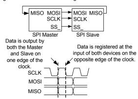
A device can be a master or slave. A master outputs clock and data to the **slave device** and inputs slave data. A slave device inputs clock and data from the master device and outputs data for input to the master. Together, the master and slave are essentially a circular Shift register, where the master generates the clocking and initiates data transfers.
