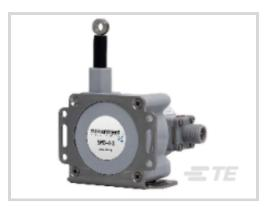
Position Sensor Product Type: SP Series, String Pots Full Stroke Range: 101.6 - 1270 mm [4 - 50 in ] Output Signal Type: 0 - 10 VDC, 4 - 20 mA Accuracy: ±.25 % of FS Repeatability: .02 % of FS
