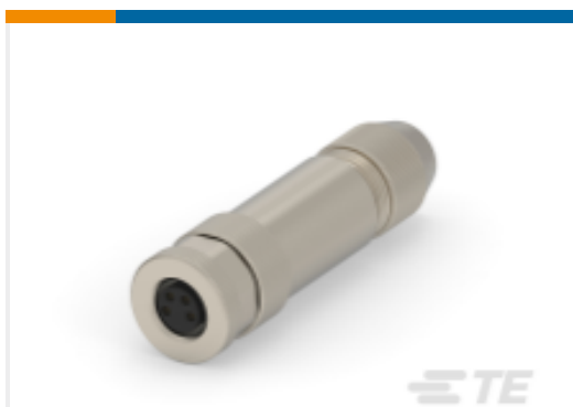
TE Part # T4010019041-000 M8,SCREW, FEMALE,S,SHIELD,4P, GOLD
