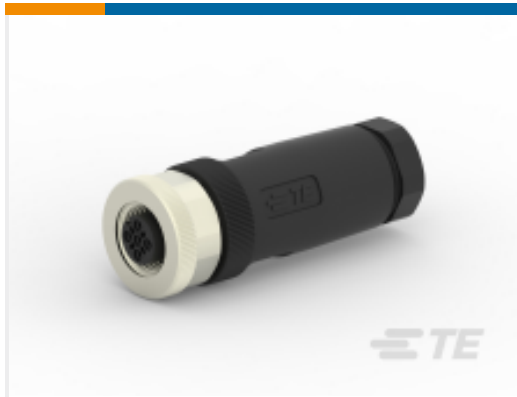
TE Part # T4110002051-000 M12,FEMALE,STRAIGHT,A CODE,5P, PG9,GOLD
