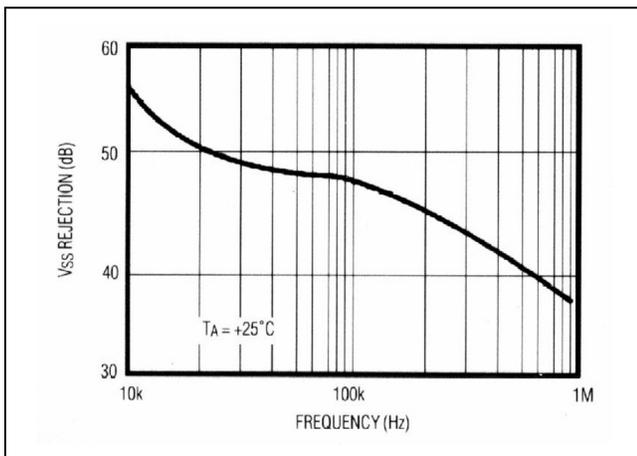
Figure 15. V<sub>SS</sub> Power-Supply Rejection vs. Frequency
