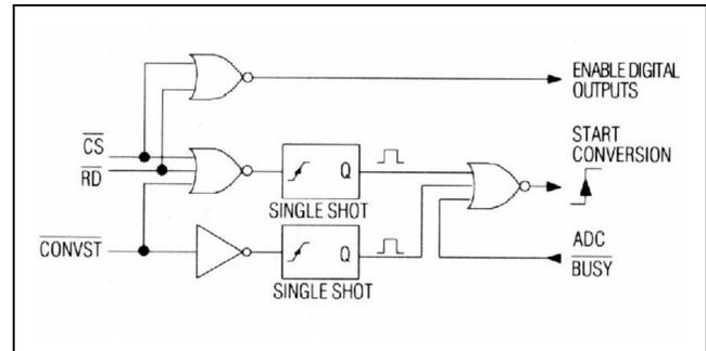
Figure 12. Conversion-Control Logic
