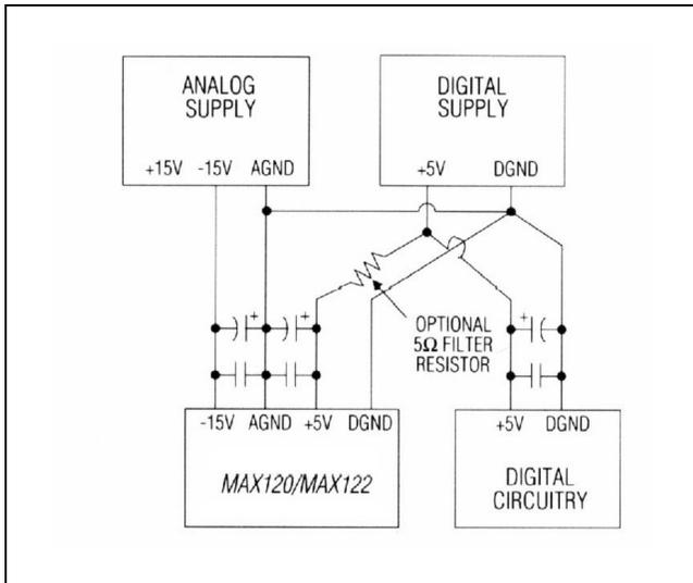
Figure 14. Power-Supply Grounding
