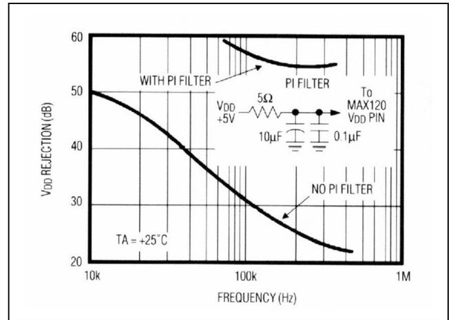
Figure 16. V<sub>DD</sub> Power-Supply Rejection vs. Frequency
