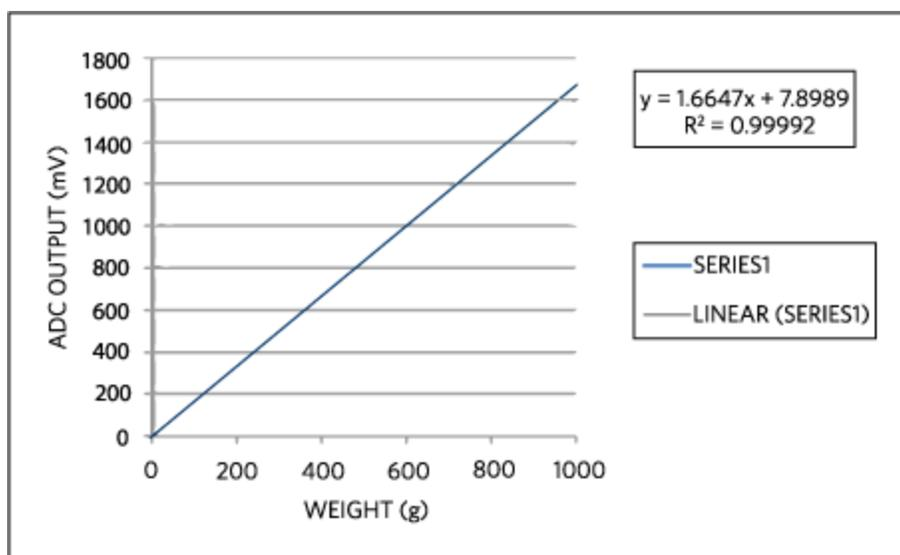
Figure 4. Load cell transferfunction with a higher dynamic range.
