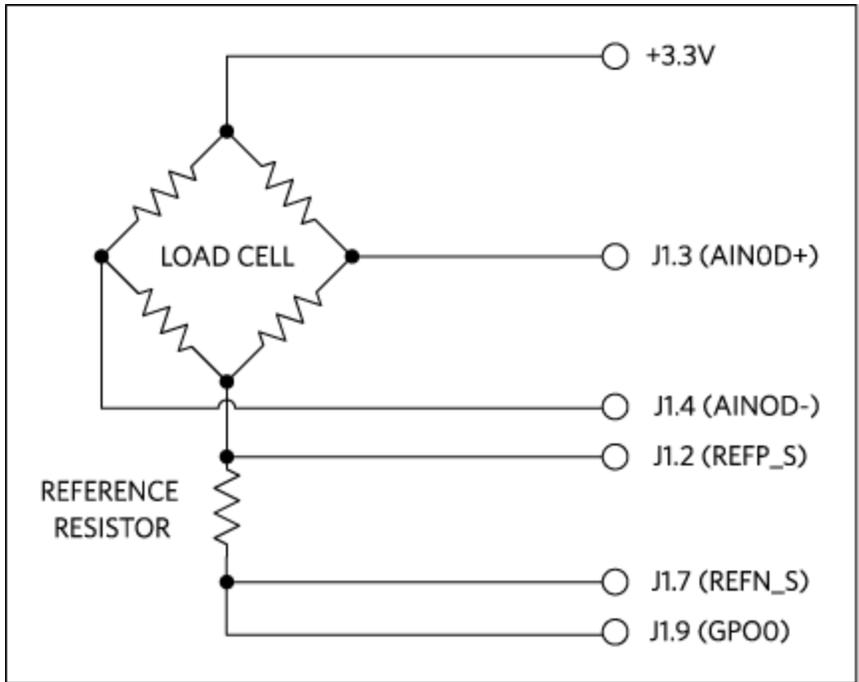
Figure 1. Weight scale Wheatstone bridge connection.
