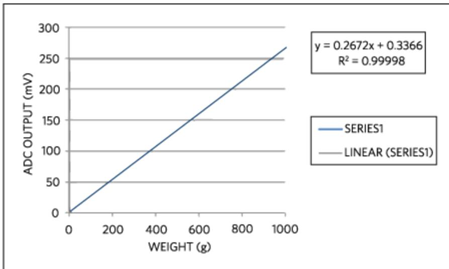
Figure 3. Transfer function of load cell.
