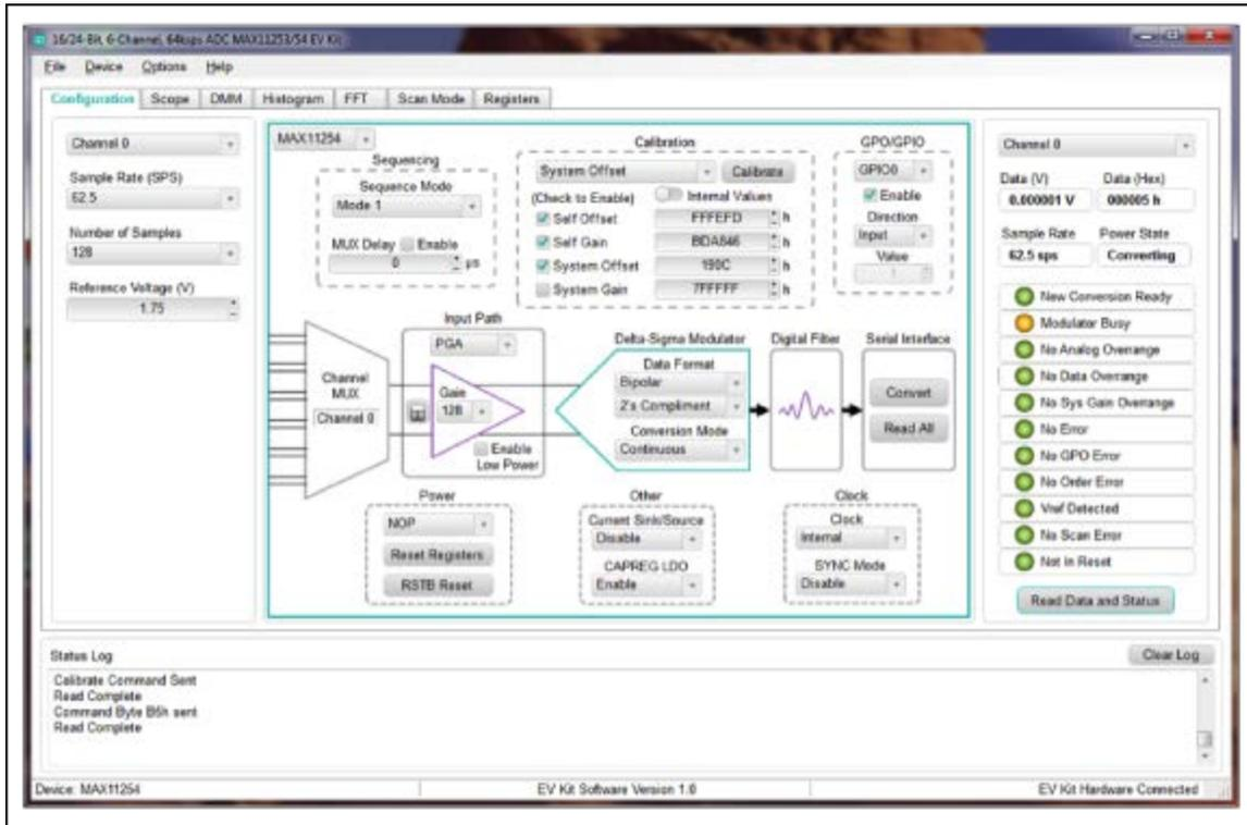
Figure 2. MAX11254 GUI setup.
