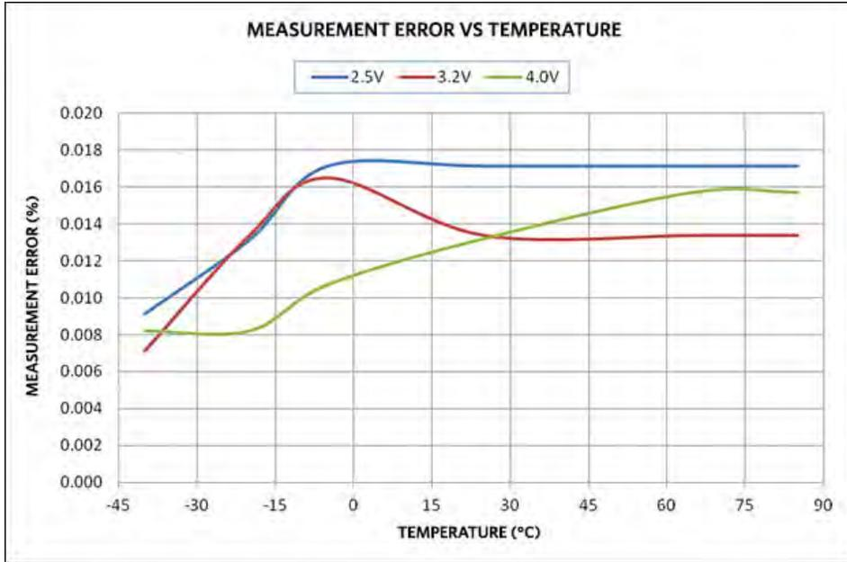
Figure 3. MAX14921 system measurement error over temperature.
