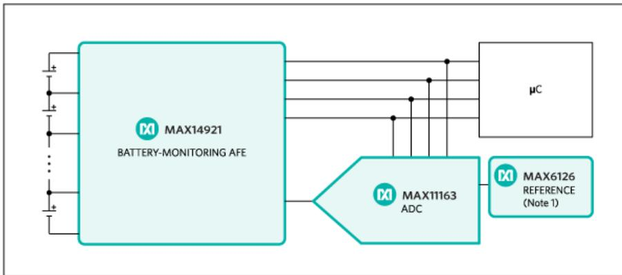
Figure 2. Maxim's evaluation kit solution for the MAX14921.
