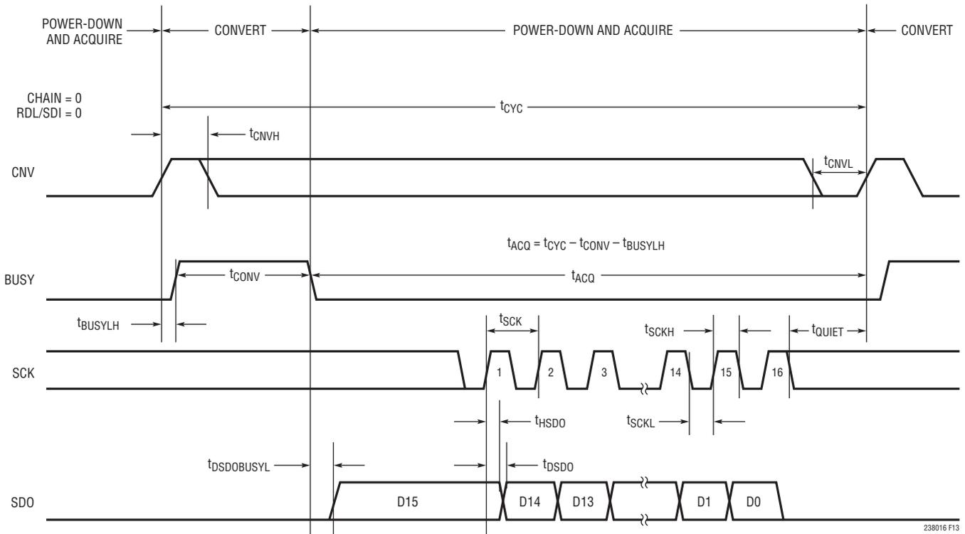
Figure 13. Using a Single LTC2380-16 in Normal Mode
