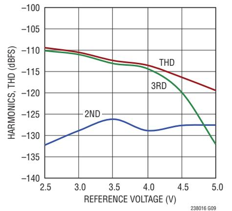
**TYPICAL PERFORMANCE CHARACTERISTICS**  $T_A = 25^\circ\text{C}$ ,  $V_{DD} = 2.5\text{V}$ ,  $0V_{DD} = 2.5\text{V}$ ,  $V_{CM} = 2.5\text{V}$ ,  $REF = 5\text{V}$ ,  $f_{SAMPL} = 2\text{MSPS}$ , unless otherwise noted.
