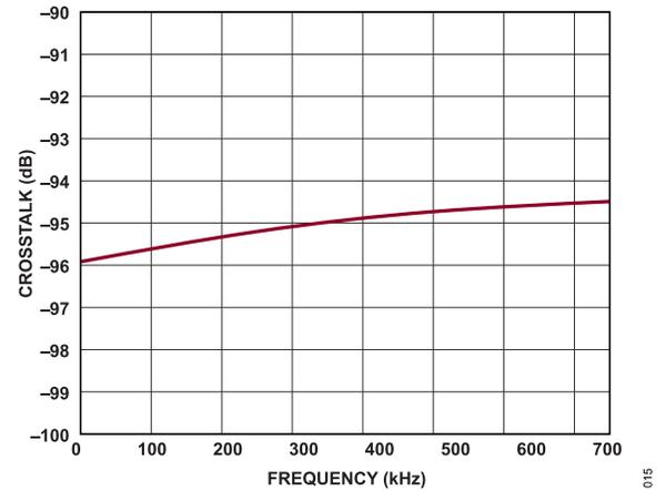
Figure 20. Crosstalk vs. Input Frequency
