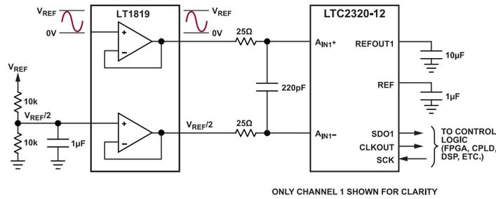
Figure 30. Pseudo-Differential Bipolar Application Circuit
