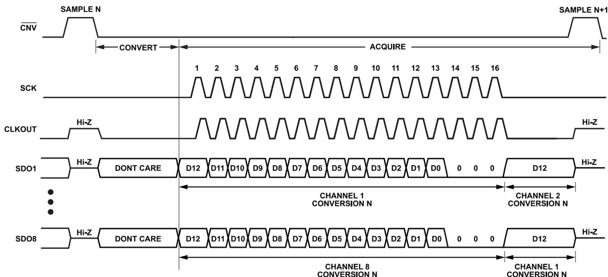
Figure 5. SDR Mode, CMOS (Reading 1 Channel per SDO)
