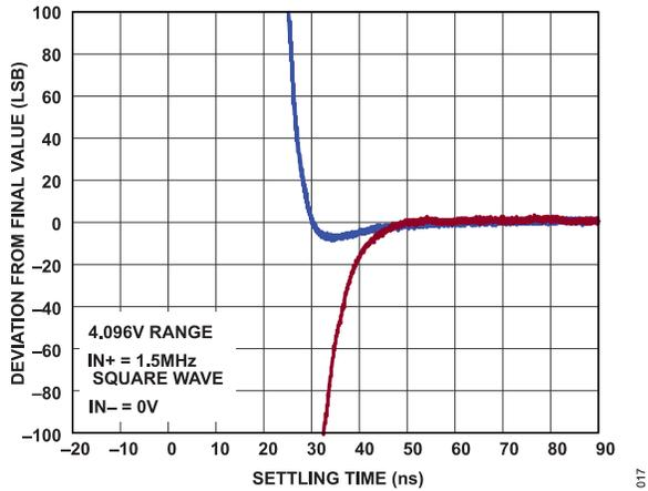
Figure 22. Step Response (Fine Settling)
