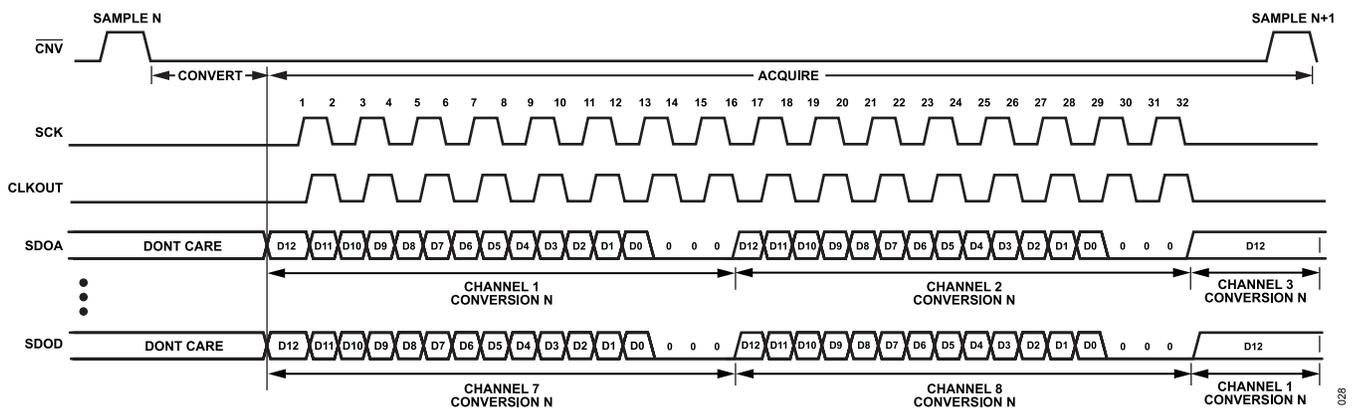
Figure 8. DDR Mode, LVDS (Reading 2 Channels per SDO Pair)
