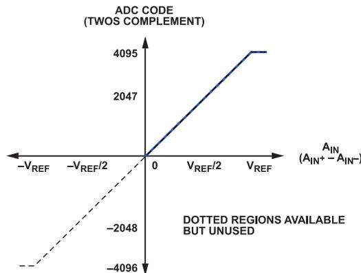
Figure 33. Pseudo-Differential Unipolar Transfer Function
