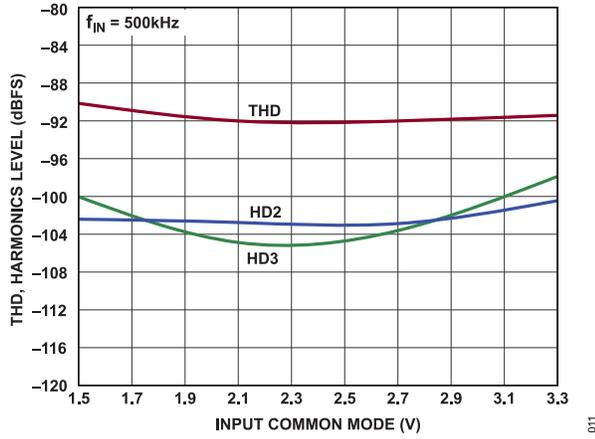
Figure 16. THD, Harmonics vs. Input Common Mode
