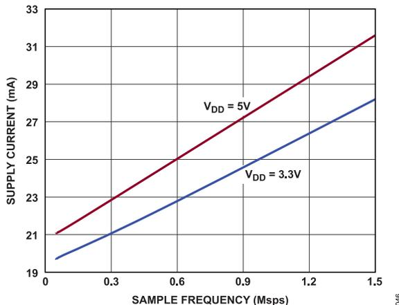
Figure 45. Power Supply Current of the LTC2320-12 Versus Sampling Rate
