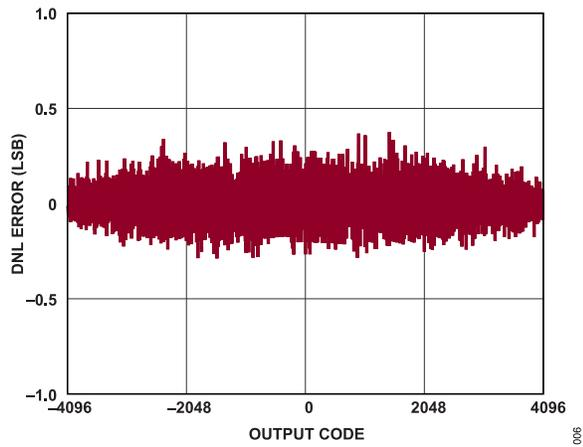
Figure 11. Differential Nonlinearity vs. Output Code
