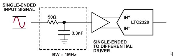
Figure 38. Input Signal Chain
