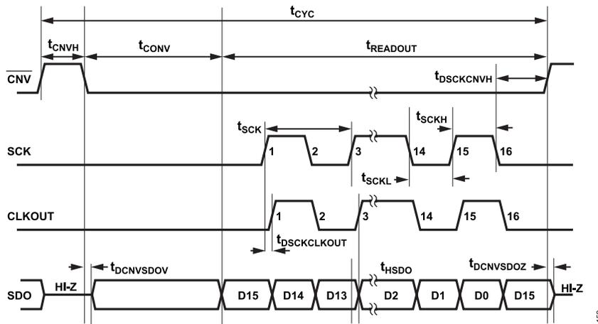
Figure 50. LTC2320-12 Timing Diagram (DDR Mode Timing)
