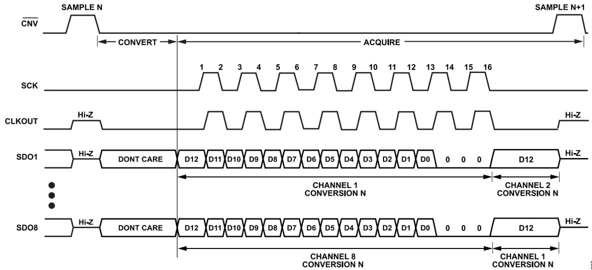
Figure 6. DDR Mode, CMOS (Reading 1 Channel per SDO)
