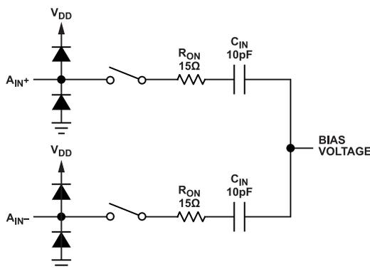
Figure 29. The Equivalent Circuit for the Differential Analog Input of the LTC2320-12
