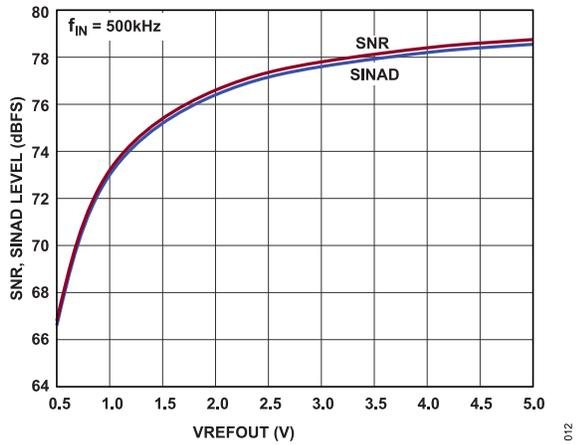
Figure 17. SNR, SINAD vs. Reference Voltage,  $f_{IN} = 500$  kHz
