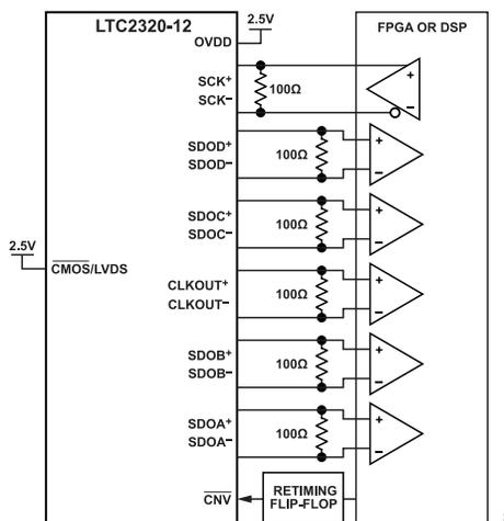
Figure 51. LTC2320-12 Using the LVDS Interface
