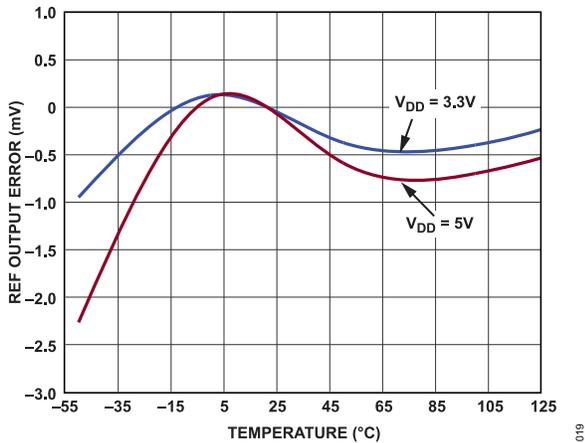
Figure 24. REF Output vs. Temperature
