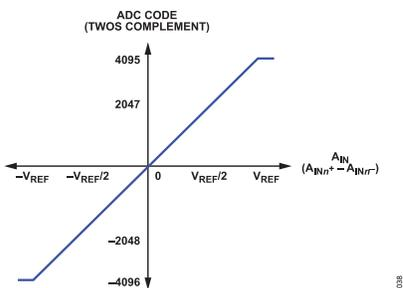
Figure 37. Fully-Differential Transfer Function
