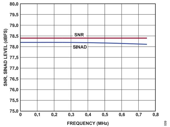
Figure 14. SNR, SINAD vs. Input Frequency (1 kHz to 750 kHz)
