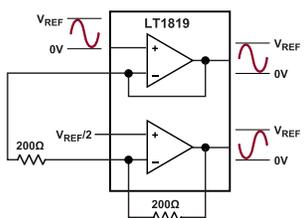
Figure 34. Single-Ended to Differential Driver
