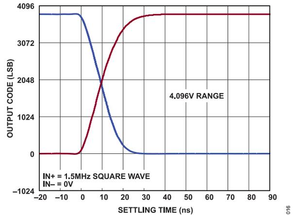
Figure 21. Step Response (Large Signal Settling)
