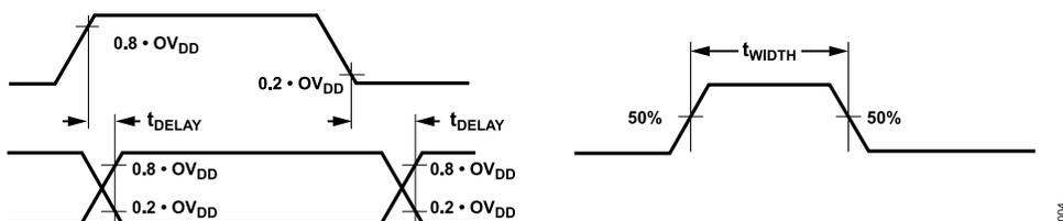
Figure 4. Voltage Levels for Timing Specifications
