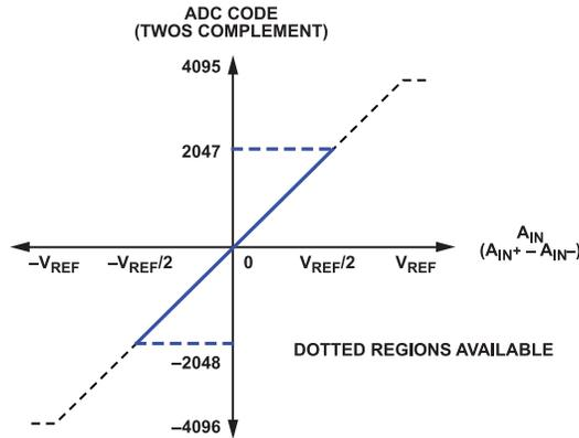
Figure 31. Pseudo-Differential Bipolar Transfer Function
