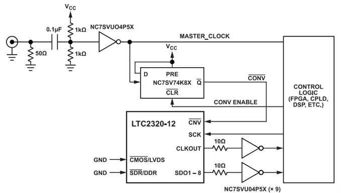
Figure 53. Low Jitter Clock Timing with RF Sine Generator Using Clock Squaring/Level-Shifting Circuit and Retiming Flip-Flop
