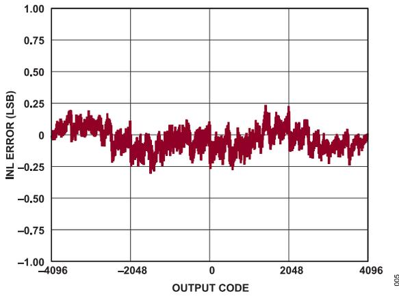
Figure 10. Integral Nonlinearity vs. Output Code
