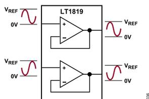
Figure 35. LT1819 Buffering a Fully-Differential Signal Source
