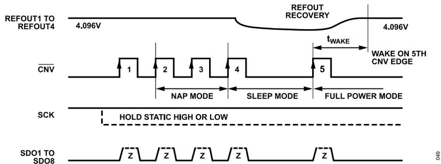
Figure 48. LVDS and CMOS Mode SLEEP and WAKE Using  $\overline{\text{CNV}}$
