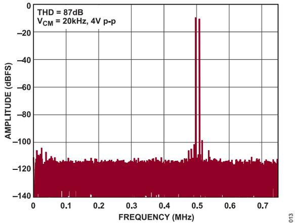
Figure 18. 32 k Point FFT, IMD,  $f_{SAMPL} = 1.5$  Msp,  $A_{IN+} = 490$  kHz,  $A_{IN-} = 510$  kHz
