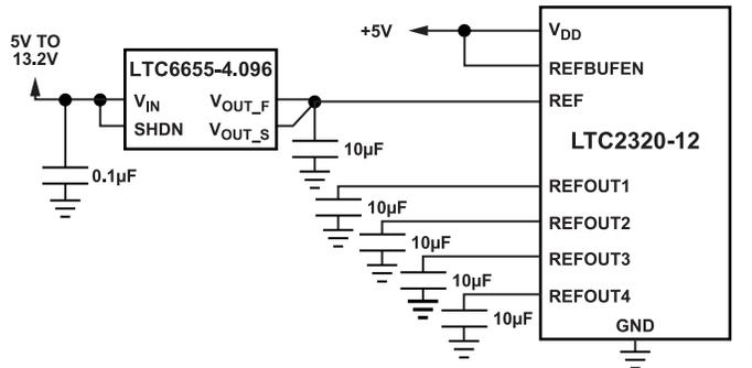
Figure 40. LTC2320-12 with a Shared External Reference Circuit
