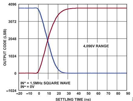
Figure 43. Transient Response of the LTC2320-12
