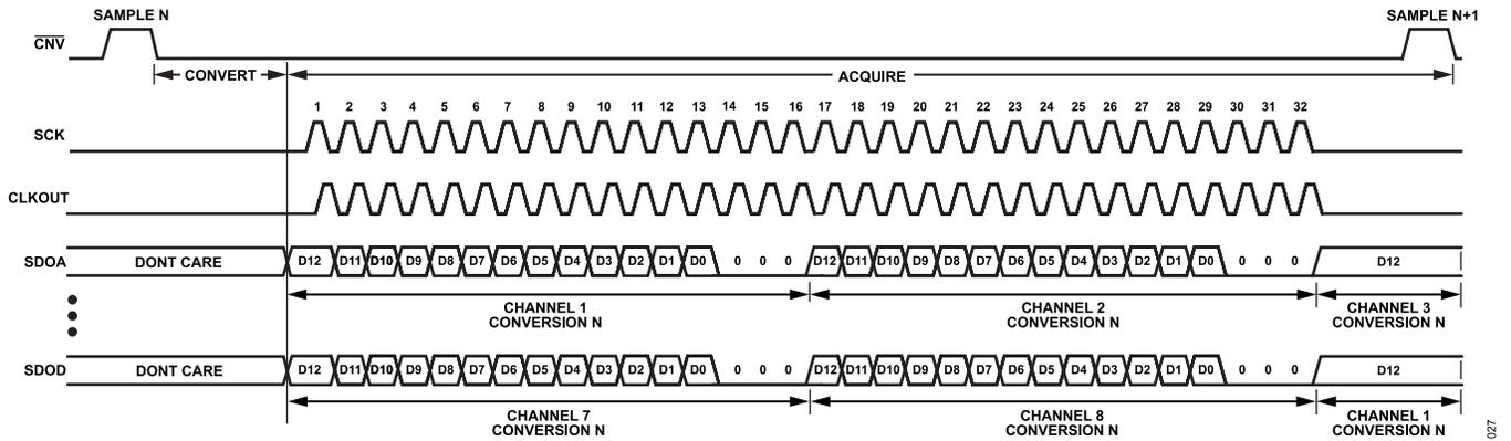
Figure 7. SDR Mode, LVDS (Reading 2 Channels per SDO Pair)
