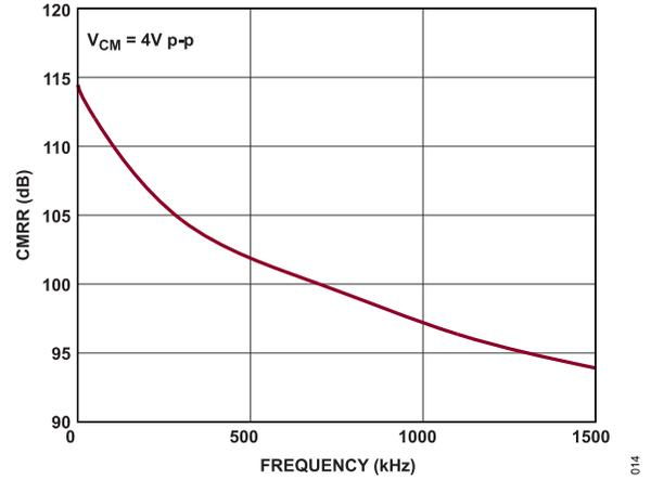
Figure 19. CMRR vs. Input Frequency
