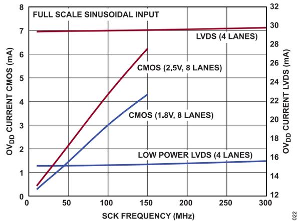
Figure 27.  $O_{VD}$  Current vs. SCK Frequency,  $C_{LOAD} = 10 pF$
