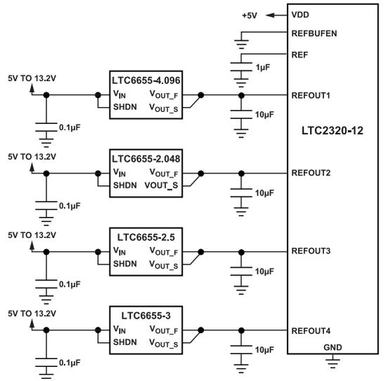
Figure 41. LTC2320-12 with Different External Reference Voltages
