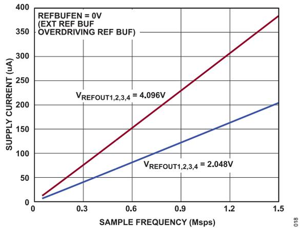
Figure 23. External Reference Supply Current vs. Sample Frequency
