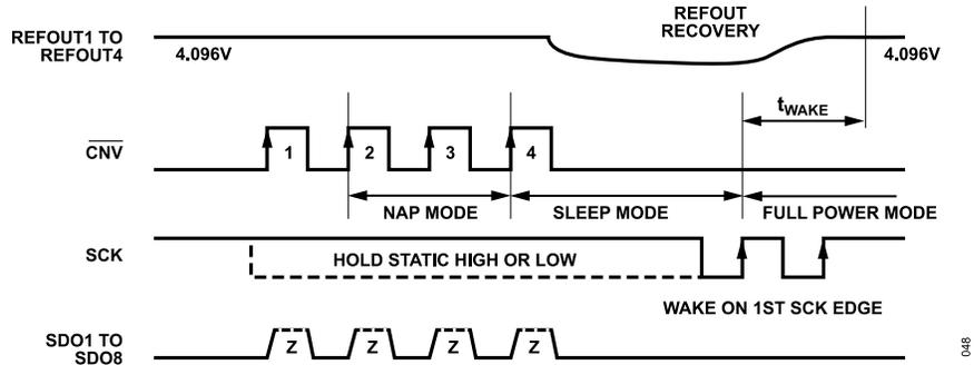
Figure 47. CMOS Mode SLEEP and WAKE Using SCK
