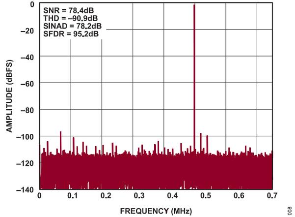
Figure 13. 32 k Point FFT,  $f_{\text{SAMPL}} = 1.5\text{ Mps}$ ,  $f_{\text{IN}} = 500\text{ kHz}$
