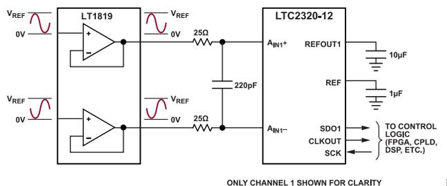
Figure 36. Fully-Differential Application Circuit
