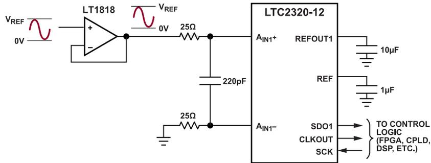
Figure 32. Pseudo-Differential Unipolar Application Circuit
