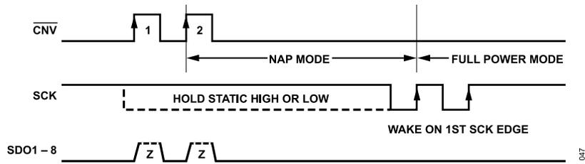
Figure 46. CMOS and LVDS Mode NAP and WAKE Using SCK
