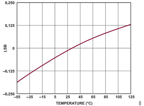
Figure 25. Offset Error vs. Temperature
