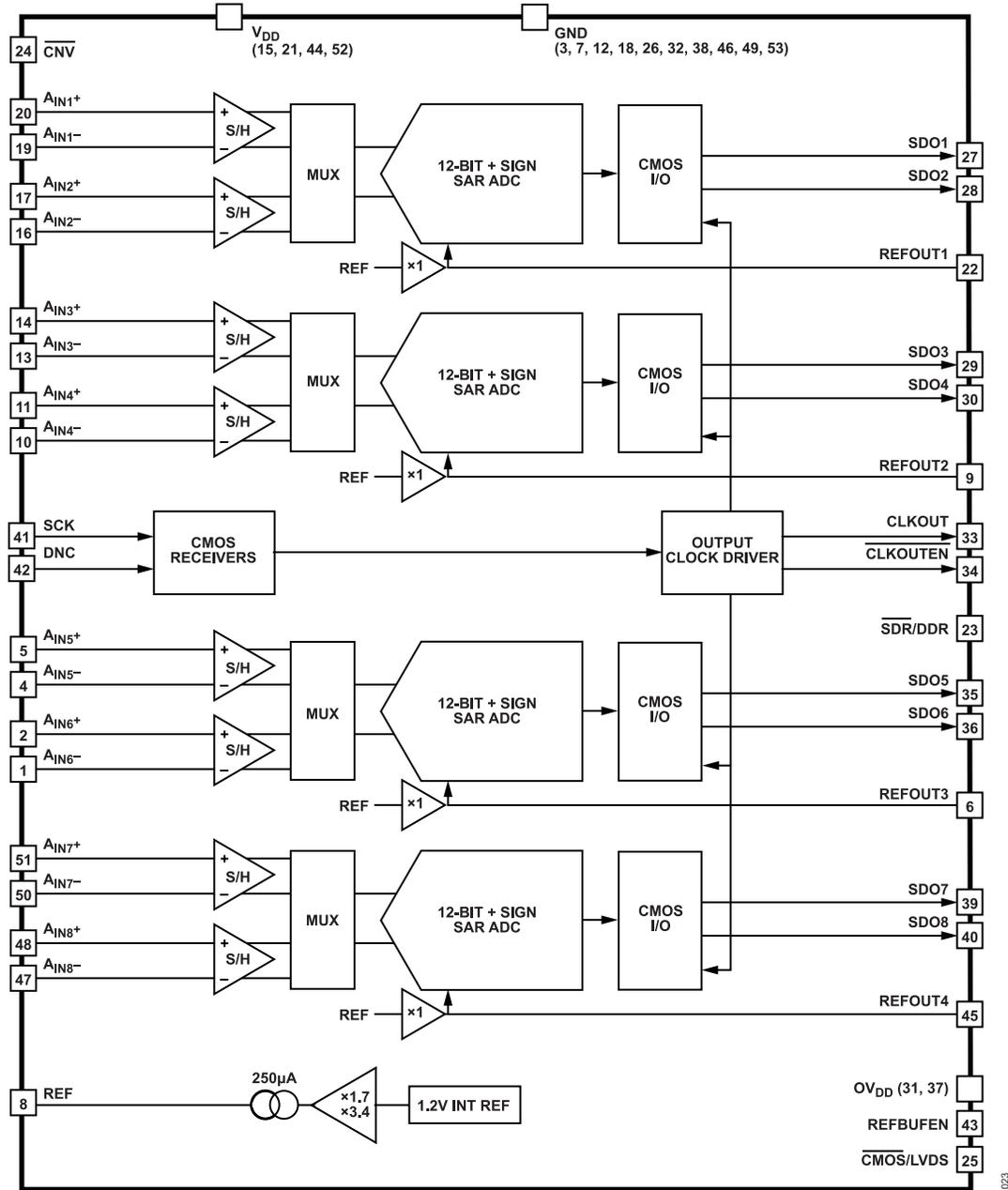
Figure 2. CMOS IO Mode
