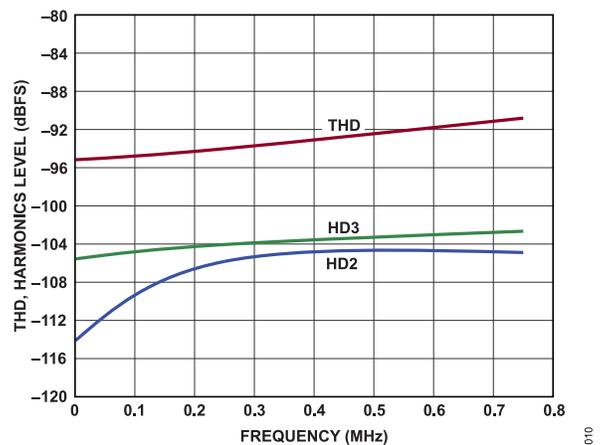
Figure 15. THD, Harmonics vs. Input Frequency (1 kHz to 750 kHz)
