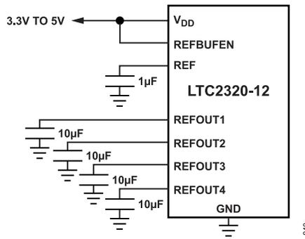
Figure 39. LTC2320-12 Internal Reference Circuit
