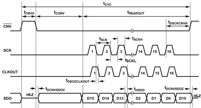
Figure 49. LTC2320-12 Timing Diagram (SDR Mode Timing)
