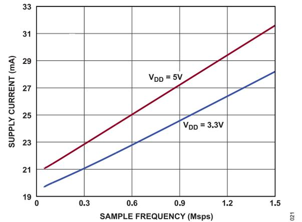
Figure 26. Supply Current vs. Sample Frequency
