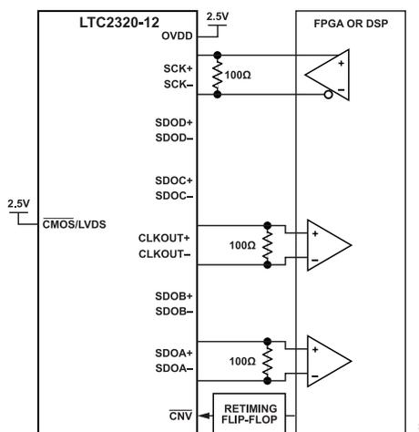
Figure 52. LTC2320-12 Using the LVDS Interface with One Lane
