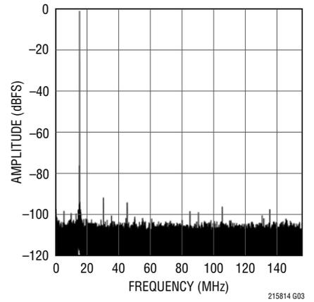
**LTC2158-14: 32K Point FFT,  $f_{IN} = 70\text{MHz}$ ,  $-1\text{dBFS}$ , 310Mps**
