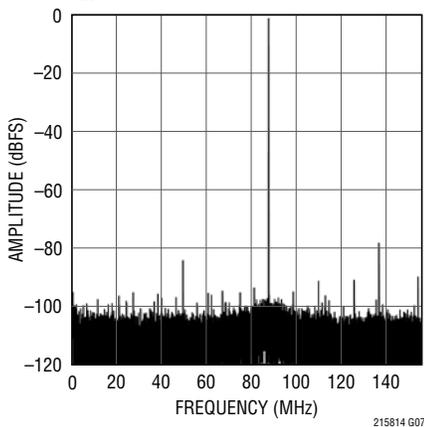
**LTC2158-14: 32K Point FFT,  $f_{IN} = 383\text{MHz}$ ,  $-1\text{dBFS}$ , 310Mps**
