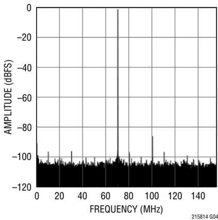
**LTC2158-14: 32K Point FFT,  $f_{IN} = 150\text{MHz}$ ,  $-1\text{dBFS}$ , 310Mps**
