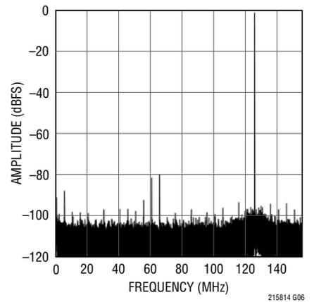
**LTC2158-14: 32K Point FFT,  $f_{IN} = 223\text{MHz}$ ,  $-1\text{dBFS}$ , 310Mps**
