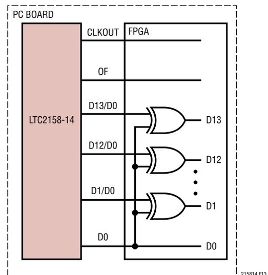
**Figure 13. Decoding a Randomized Digital Output Signal**
