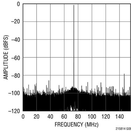
**LTC2158-14: 32K Point FFT,  $f_{IN} = 421\text{MHz}$ ,  $-1\text{dBFS}$ , 310Mps**
