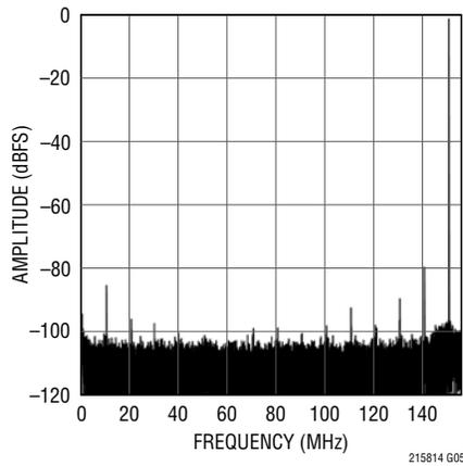
**LTC2158-14: 32K Point FFT,  $f_{IN} = 185\text{MHz}$ ,  $-1\text{dBFS}$ , 310Mps**
