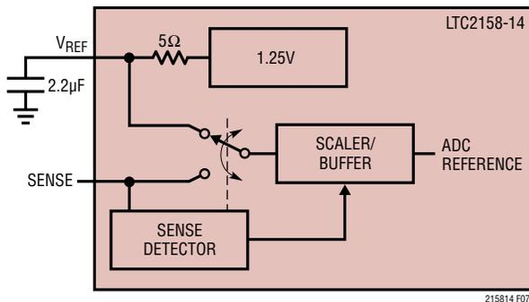
Figure 7. Reference Circuit
