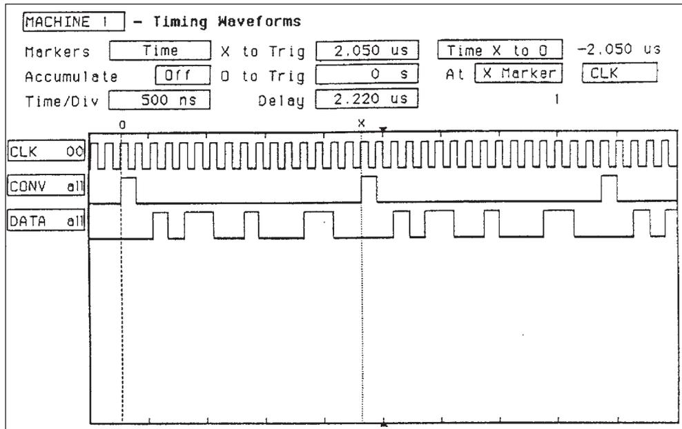
NOTE: THE TMS320C50-40MHz HAS A LIMITED SERIAL PORT CLOCK SPEED OF 7.8MHz. TO ALLOW THE LTC1404 TO RUN AT ITS MAXIMUM SPEED OF 9.6MHz, THE TMS320C50-57 OR TMS320C50-80MHz IS NEEDED
