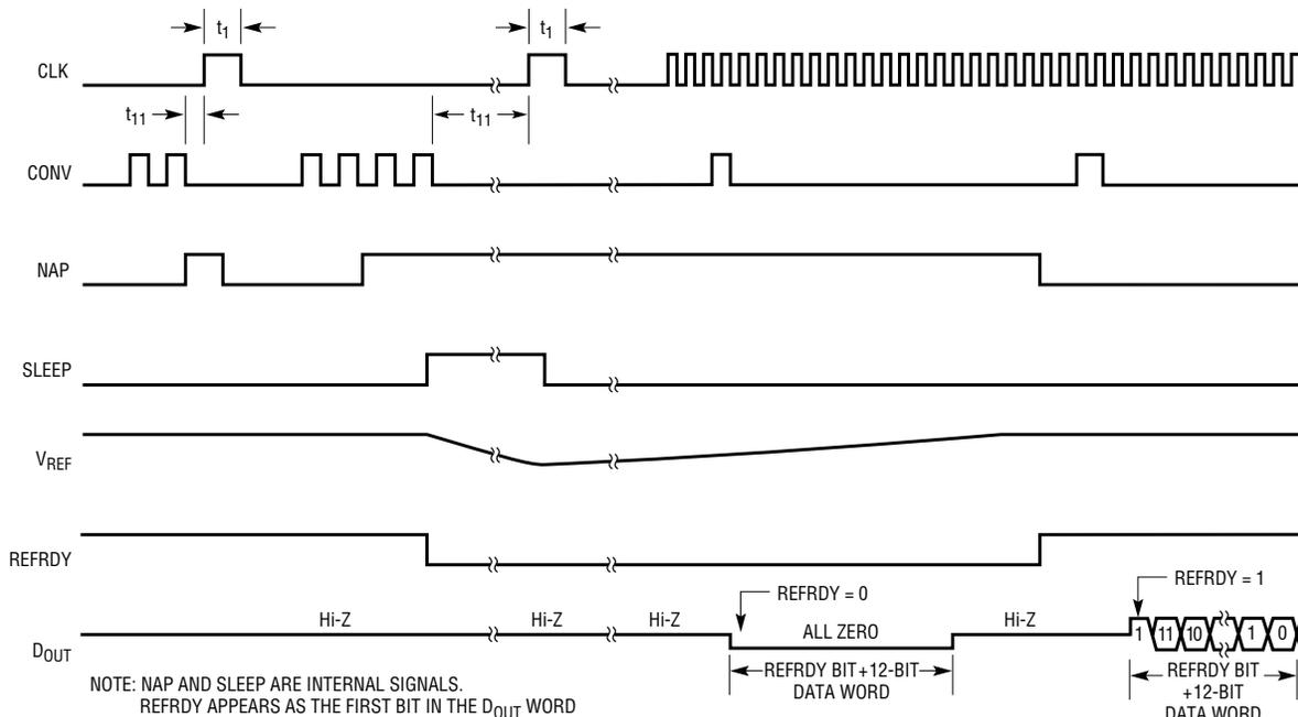
Figure 12. Nap Mode and Sleep Mode Waveforms
