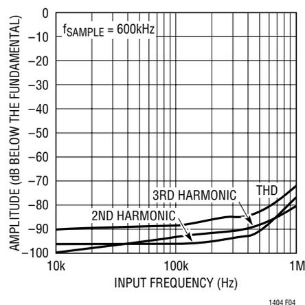
Figure 4. Distortion vs Input Frequency in Bipolar Mode
