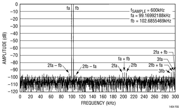
Figure 5. Intermodulation Distortion Plot in Bipolar Mode
