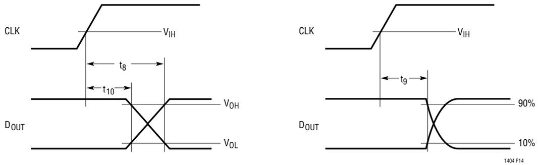
Figure 14. CLK to D<sub>OUT</sub> Delay
