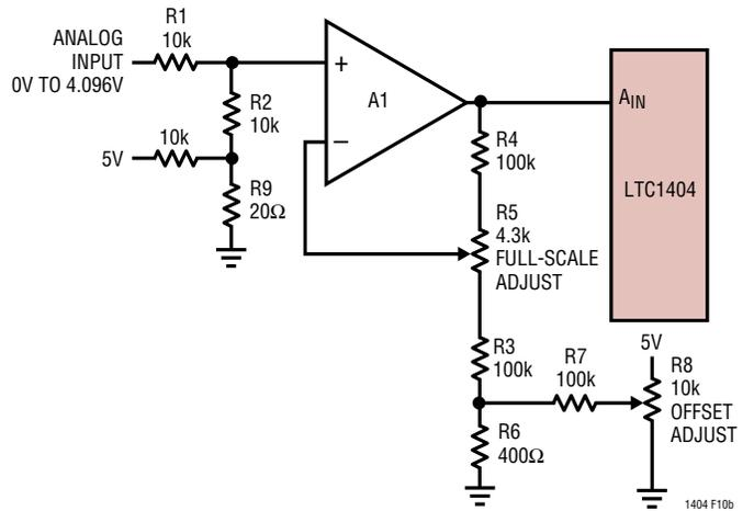
Figure 10b. LTC1404 Offset and Full-Scale Adjust Circuit
