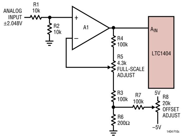
Figure 10c. LTC1404 Bipolar Offset and Full-Scale Adjust Circuit
