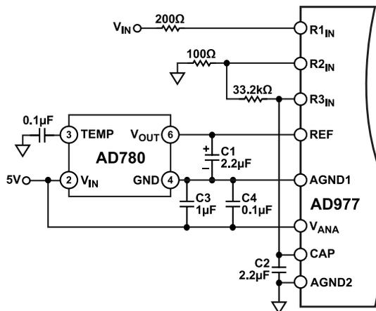
Figure 19. AD780 External Reference to AD977 Configured for ±10 V Input Range
