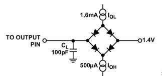
Figure 2. Load Circuit for Digital Interface Timing
