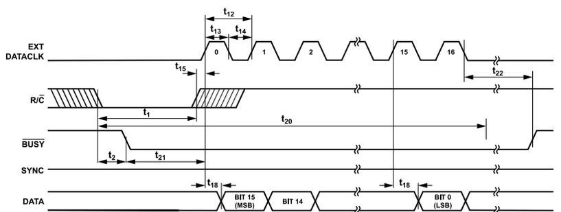
Figure 8. Conversion and Read Timing for Reading Previous Conversion Results During A Conversion Using External Discontinuous Data Clock ( $\overline{\text{EXT}}/\overline{\text{INT}}$  Set to Logic High,  $\overline{\text{CS}}$  Set to Logic Low)
