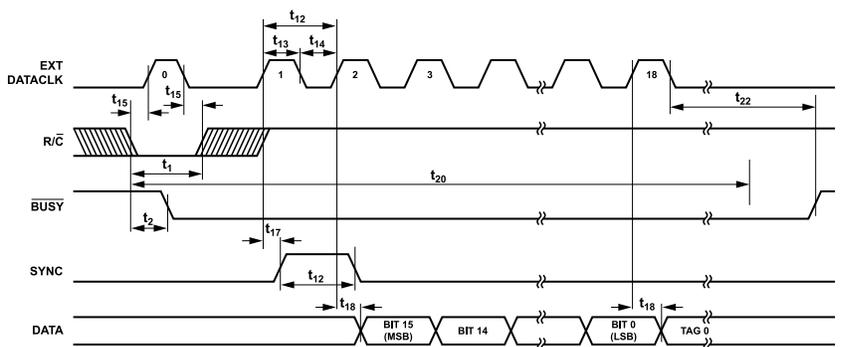
Figure 10. Conversion and Read Timing for Reading Previous Conversion Results During a Conversion Using External Discontinuous Data Clock ( $\overline{\text{EXT}}/\overline{\text{INT}}$  Set to Logic High, CS Set to Logic Low)
