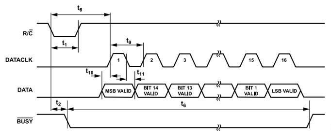
Figure 6. Serial Data Timing for Reading Previous Conversion Results with Internal Clock ( $\overline{CS}$ ,  $\overline{EXT}/\overline{INT}$  and TAG Set to Logic Low)
