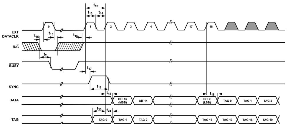
Figure 9. Conversion and Read Timing Using An External Discontinuous Data Clock (EXT/INT Set to Logic High, CS Set to Logic Low)
