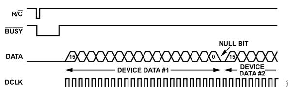
Figure 32. TAG Timing Diagram for Two Concatenated AD977/AD977As
