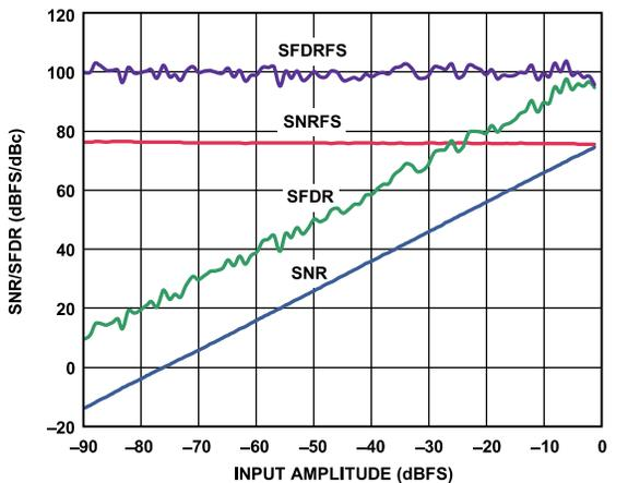
Figure 17. SNR/SFDR vs. Analog Input Level;  $f_{IN} = 9.7$  MHz,  $f_{SAMPLE} = 80$  MSPS
