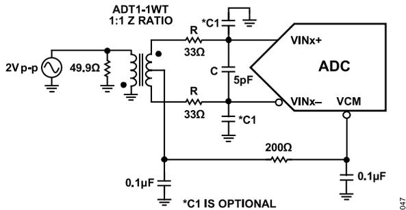
**Figure 56. Differential Transformer-Coupled Configuration for Baseband Applications**
