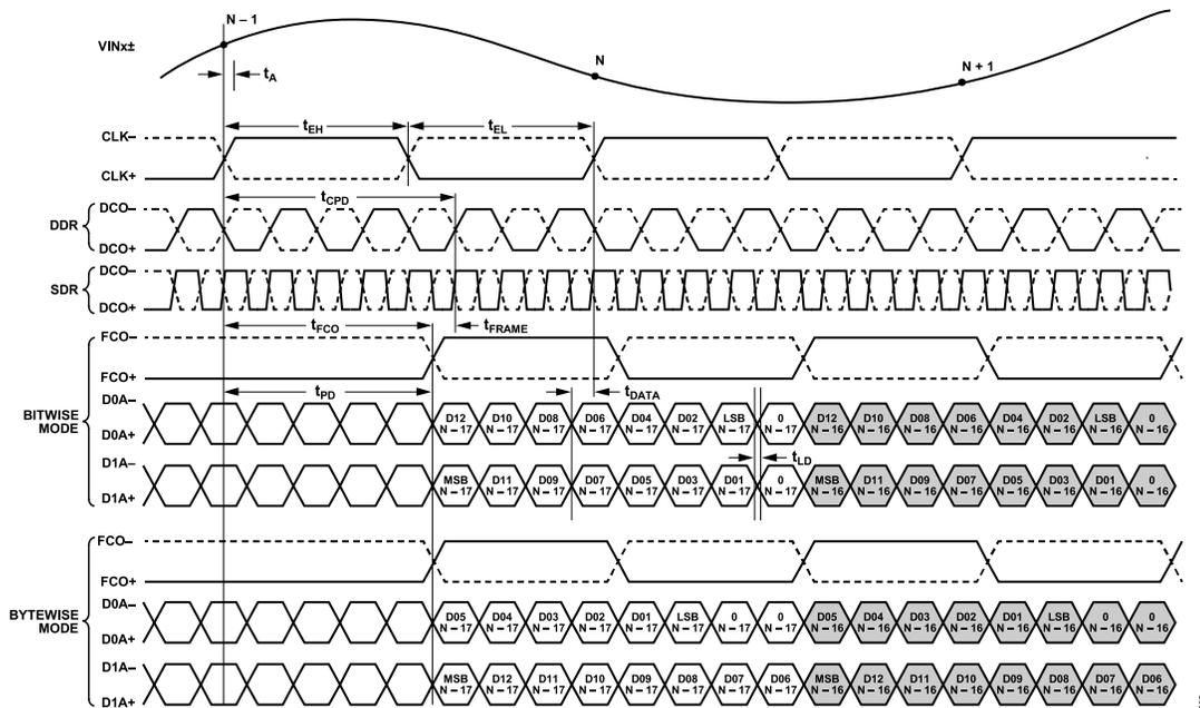
Figure 2. 16-Bit DDR/SDR, Two-Lane, 1x Frame Mode (Default)
