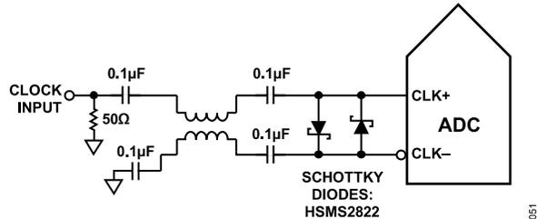
Figure 60. Balun-Coupled Differential Clock (Up to 1 GHz)
