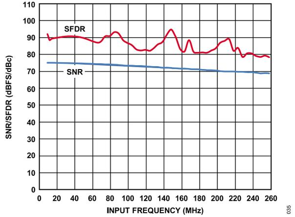
Figure 37. SNR/SFDR vs.  $f_{IN}$ ;  $f_{SAMPLE} = 125 \text{ MSPS}$
