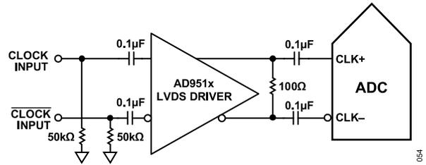
Figure 62. Differential LVDS Sample Clock (Up to 1 GHz)
