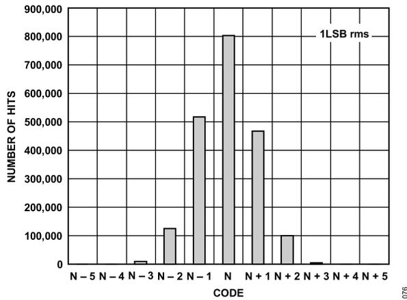
Figure 41. Input Referred Noise Histogram;  $f_{SAMPLE} = 125 \text{ MSPS}$
