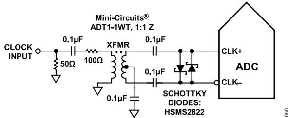
Figure 59. Transformer-Coupled Differential Clock (Up to 200 MHz)
