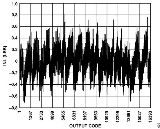
Figure 22. INL;  $f_{IN} = 9.7 \text{ MHz}$ ,  $f_{SAMPLE} = 80 \text{ MSPS}$
