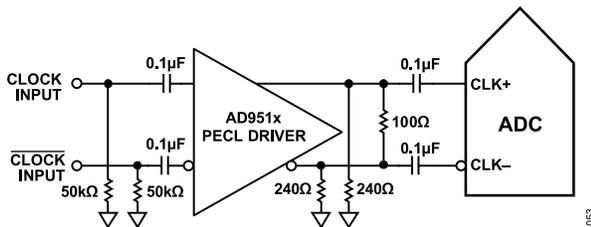
Figure 61. Differential PECL Sample Clock (Up to 1 GHz)
