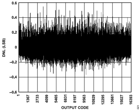
Figure 23. DNL;  $f_{IN} = 9.7 \text{ MHz}$ ,  $f_{SAMPLE} = 80 \text{ MSPS}$
