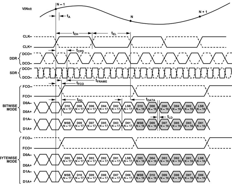
Figure 5. 12-Bit DDR/SDR, Two-Lane, 2x Frame Mode
