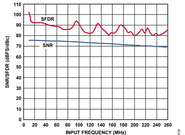
Figure 20. SNR/SFDR vs.  $f_{IN}$ ;  $f_{SAMPLE} = 80$  MSPS
