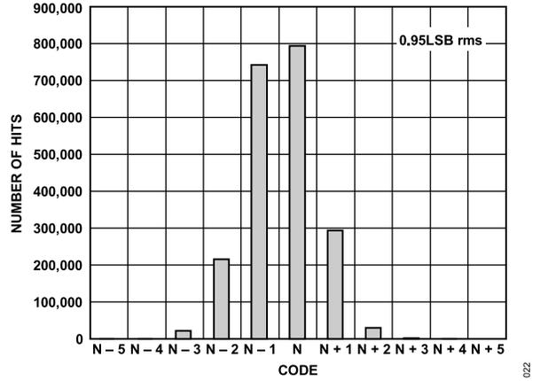
Figure 24. Input Referred Noise Histogram;  $f_{SAMPLE} = 80 \text{ MSPS}$
