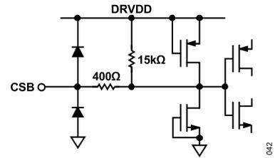
Figure 51. Equivalent CSB Input Circuit
