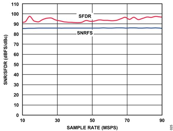
Figure 27. SNR/SFDR vs. Sample Rate;  $f_{IN} = 70$  MHz,  $f_{SAMPLE} = 80$  MSPS
