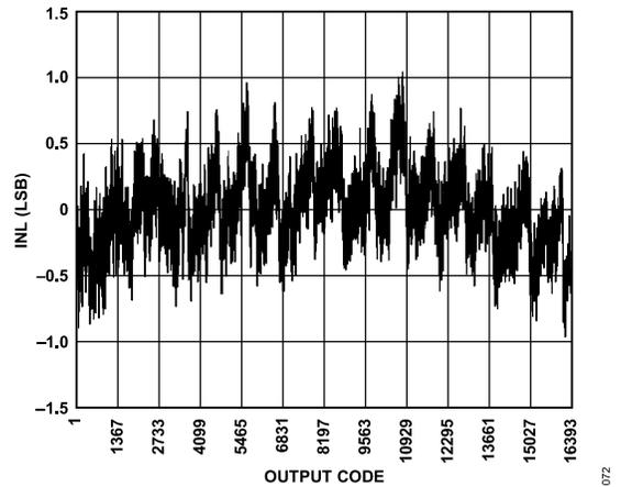
Figure 39. INL;  $f_{IN} = 9.7 \text{ MHz}$ ,  $f_{SAMPLE} = 125 \text{ MSPS}$
