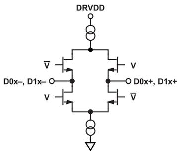
Figure 48. Equivalent Digital Output Circuit
