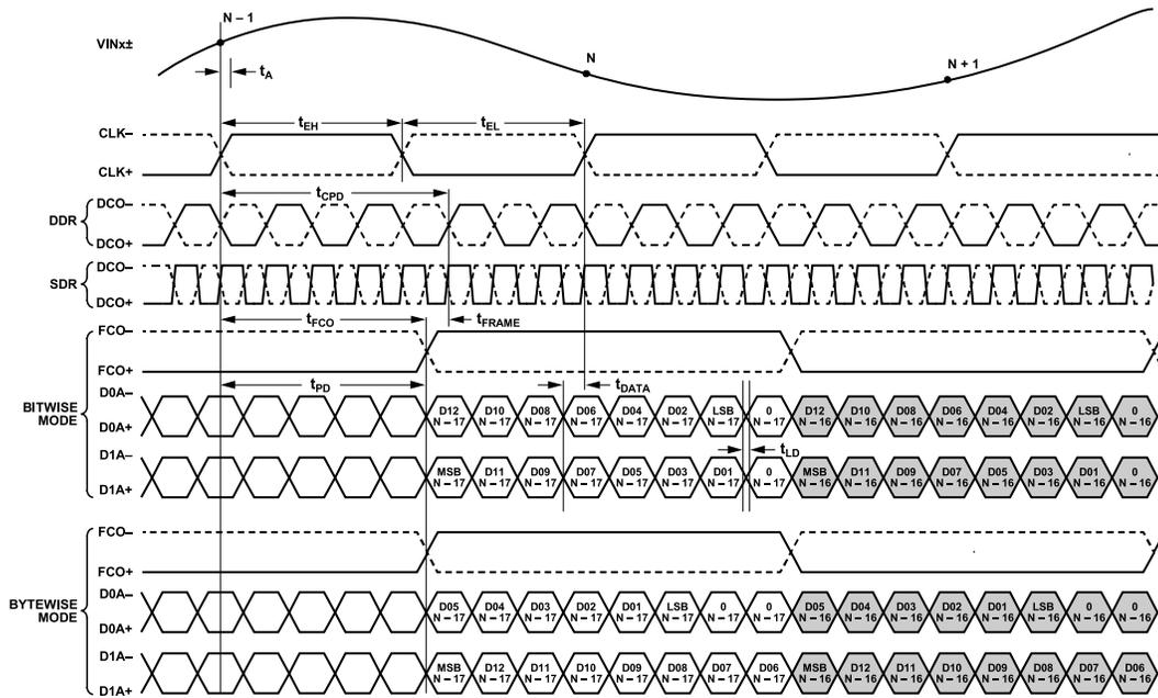
Figure 4. 16-Bit DDR/SDR, Two-Lane, 2x Frame Mode
