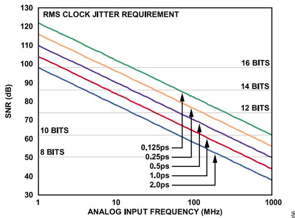
Figure 64. Ideal SNR vs. Input Frequency and Jitter
