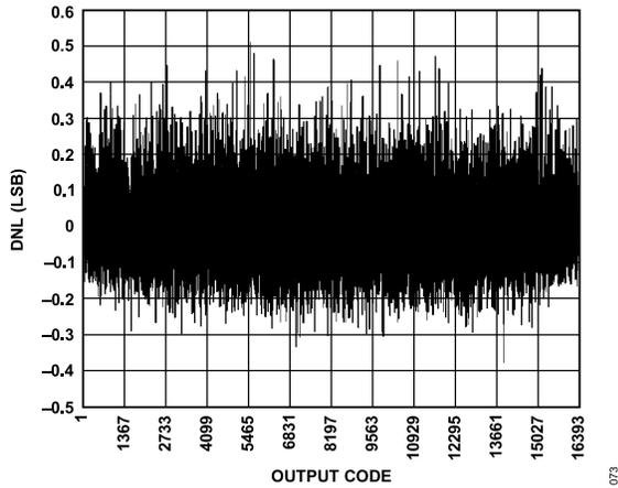
Figure 40. DNL;  $f_{IN} = 9.7 \text{ MHz}$ ,  $f_{SAMPLE} = 125 \text{ MSPS}$
