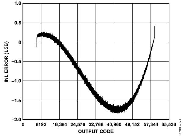
Figure 21. INL with  $f_{IN} = 2.4$  MHz
