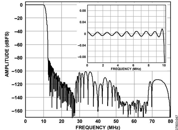
Figure 47. 10 MHz Signal Bandwidth, 160 MSPS
