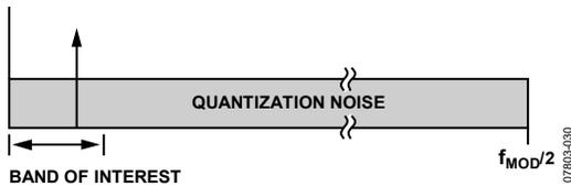
Figure 30. Quantization Noise
