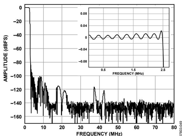
Figure 49. 2.5 MHz Signal Bandwidth, 160 MSPS
