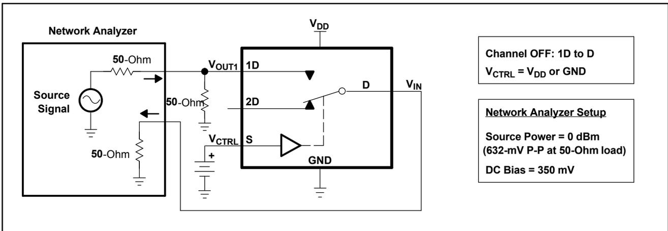
**Figure 3. OFF Isolation (O<sub>ISO</sub>)**
