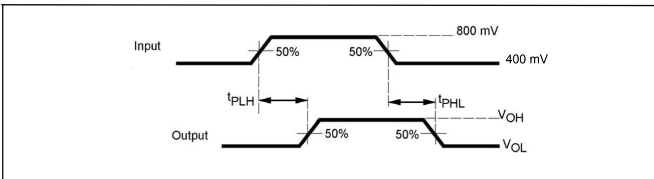
**Figure 6. Propagation Delay**
