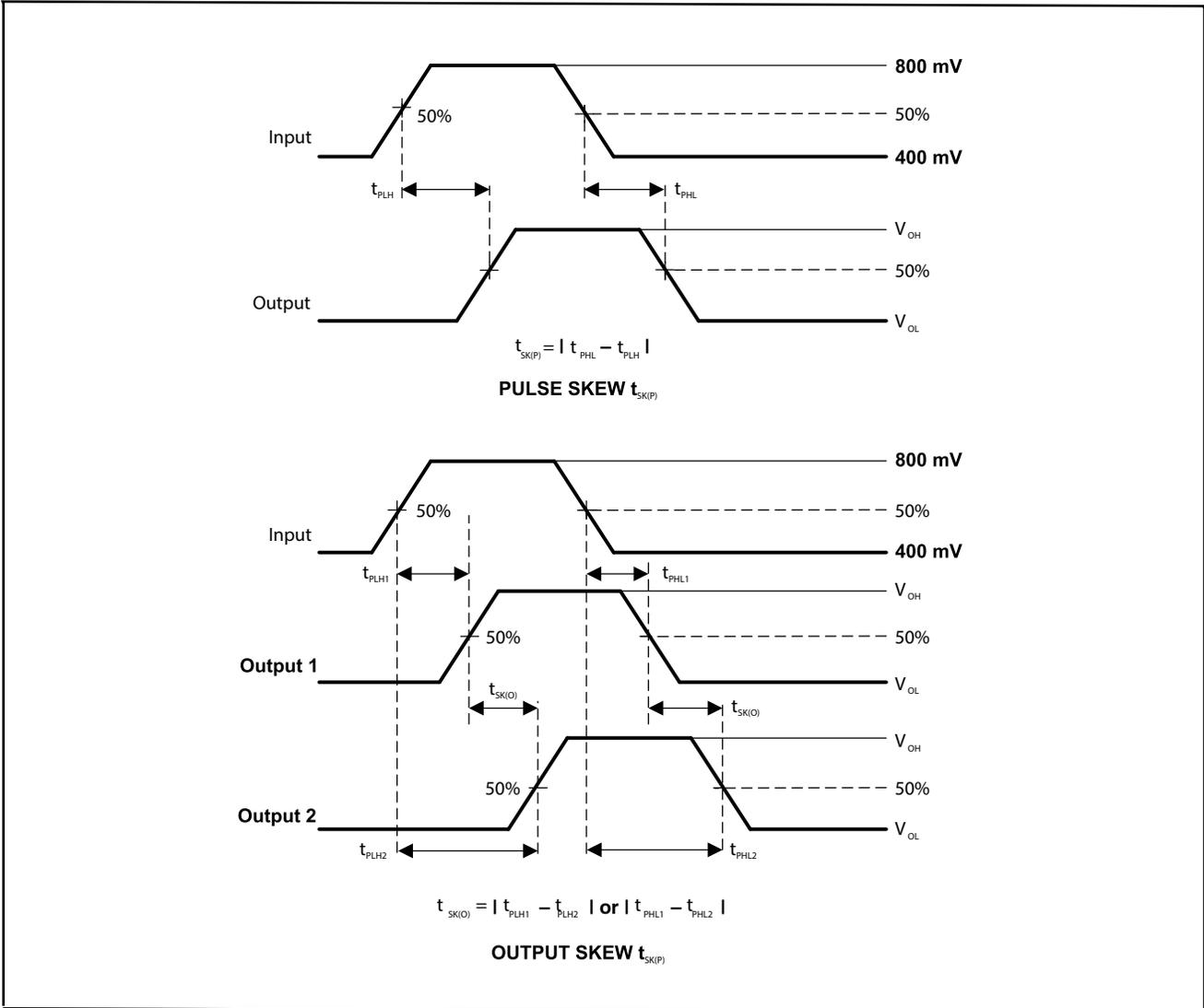
Figure 7. Skew Test
