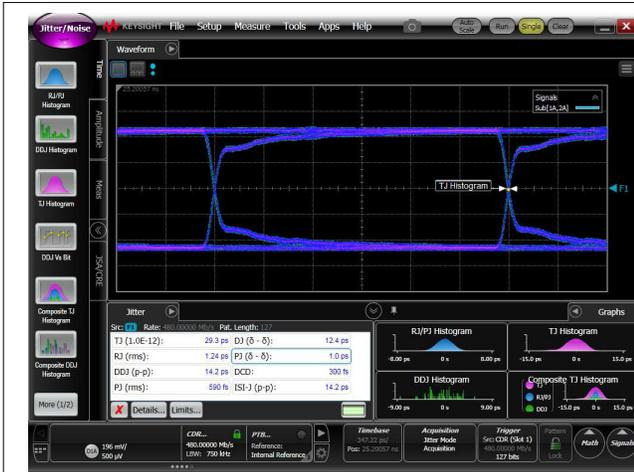
Figure 6-7. Through Calibration Traces at 480Mbps
