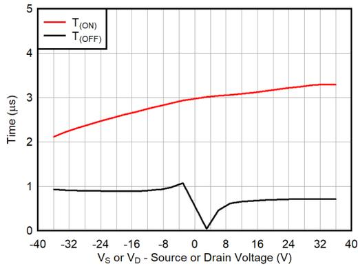
**Figure 7-27. Turn-On and Turn-Off Times vs Source Voltage**
