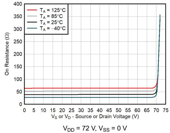
Figure 7-8. On-Resistance vs Source or Drain Voltage
