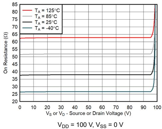
Figure 7-9. On-Resistance vs Source or Drain Voltage
