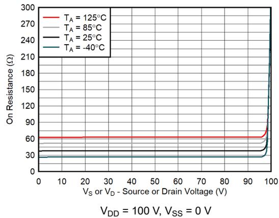
Figure 7-10. On-Resistance vs Source or Drain Voltage
