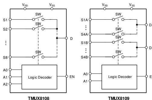
**TMUX8108 and TMUX8109 Block Diagram**
