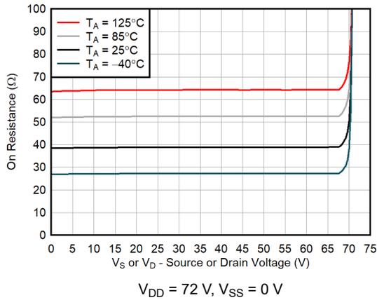
Figure 7-7. On-Resistance vs Source or Drain Voltage
