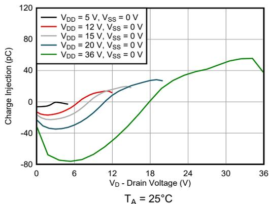
Figure 5-17. Charge Injection vs Drain Voltage – Single Supplies
