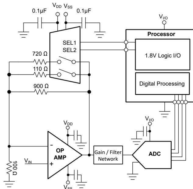
Figure 8-1. Gain Switching
