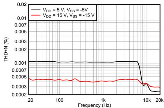
Figure 5-23. THD+N vs Frequency (Dual Supplies)
