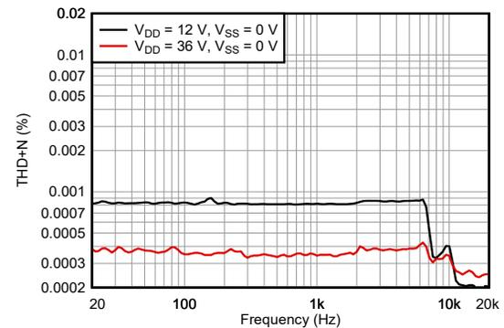
Figure 5-24. THD+N vs Frequency (Single Supplies)
