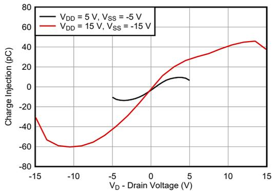
Figure 5-15. Charge Injection vs Drain Voltage – Dual Supplies
