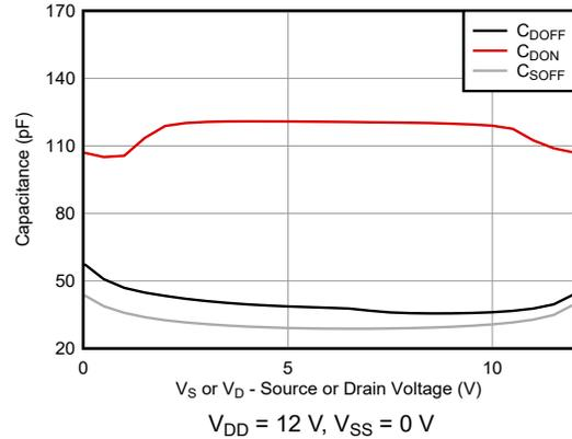
**Figure 5-28. Capacitance vs Source Voltage or Drain Voltage**
