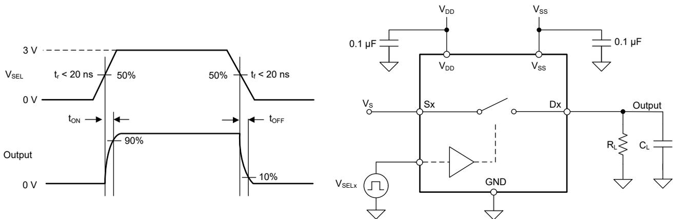
Figure 6-4. Turn-On and Turn-Off Time Measurement Setup
