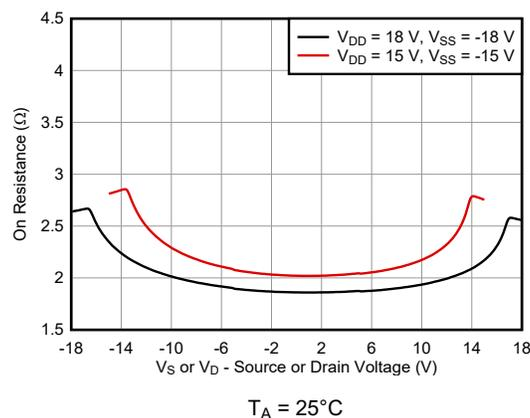
**Figure 8-2. On-Resistance vs Source or Drain Voltage**
