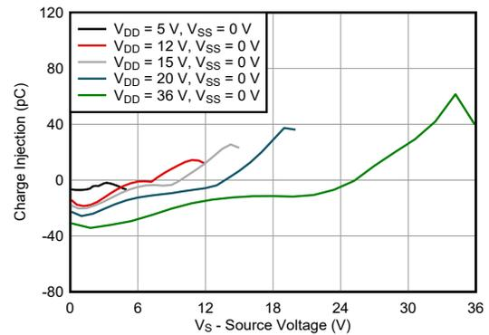
Figure 5-16. Charge Injection vs Source Voltage – Single Supplies
