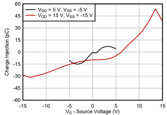
Figure 5-14. Charge Injection vs Source Voltage – Dual Supplies
