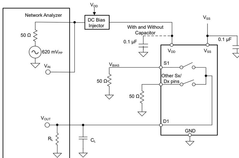
Figure 6-12. AC PSRR Measurement Setup
