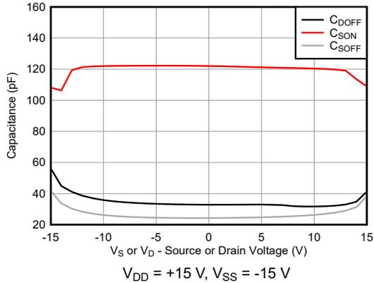
**Figure 5-27. Capacitance vs Source Voltage or Drain Voltage**
