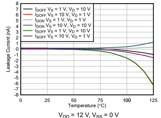
**Figure 5-12. Leakage Current vs Temperature**
