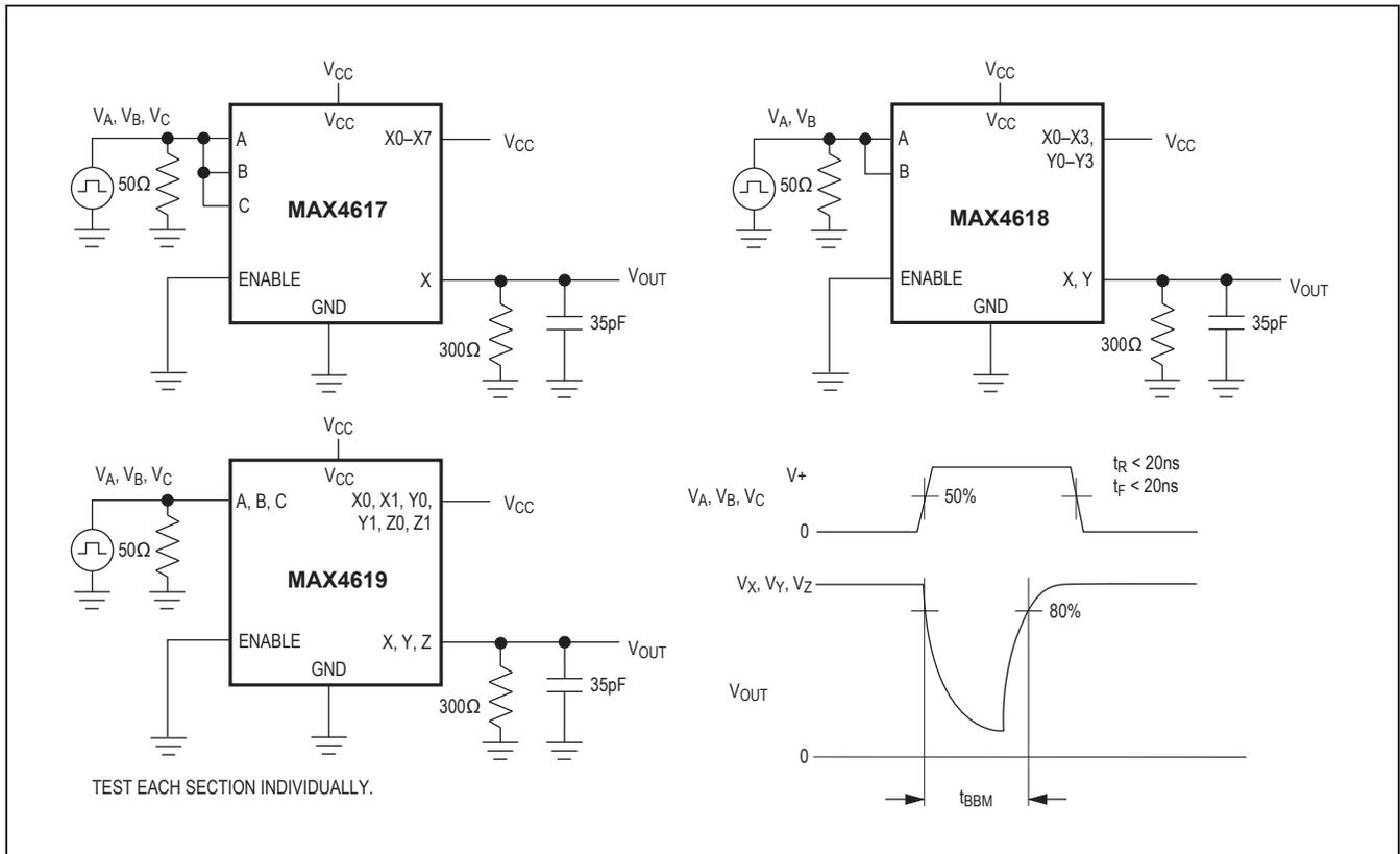
Figure 4. Break-Before-Make Interval
