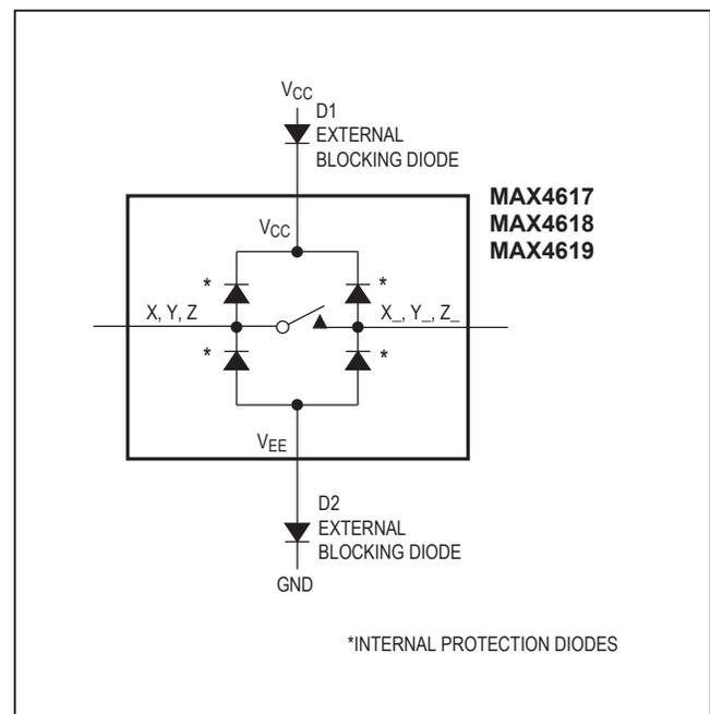
Figure 1. Overvoltage Protection Using External Blocking Diodes
