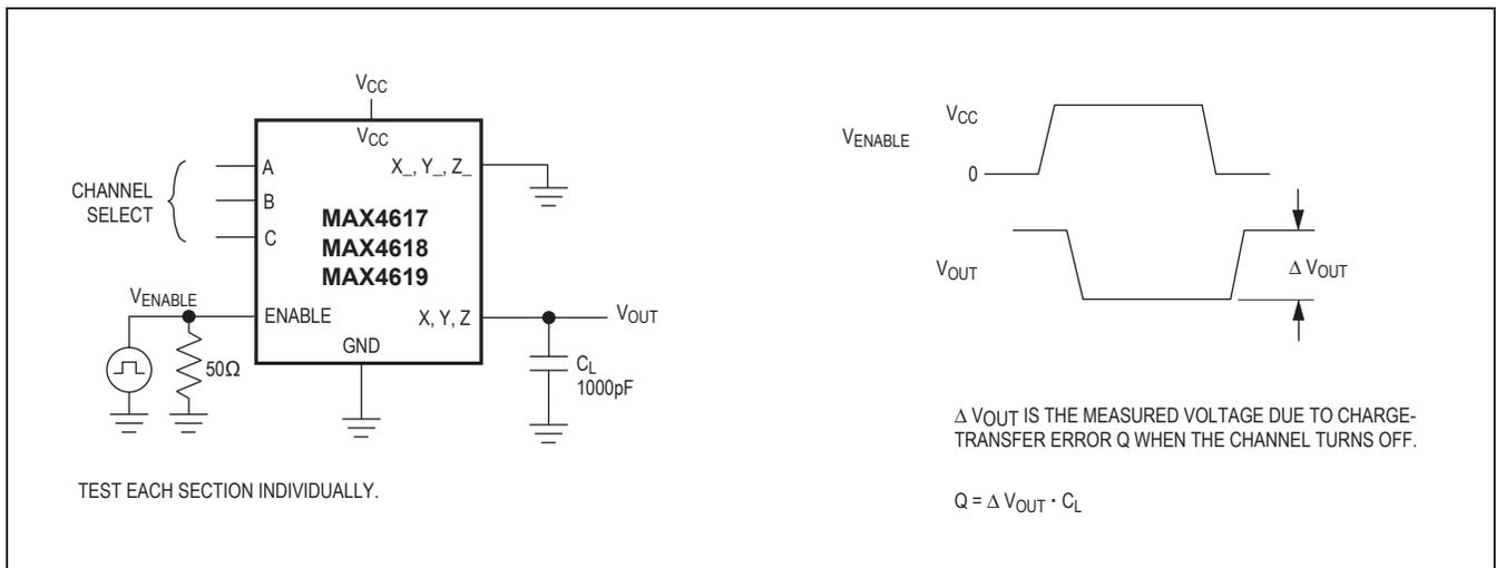
Figure 5. Charge Injection
