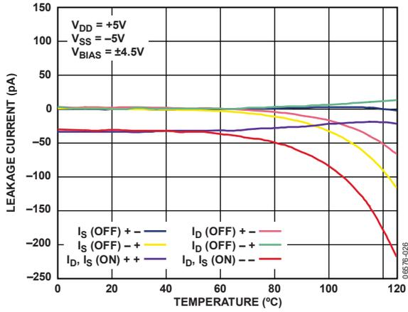
Figure 9. Leakage Currents vs. Temperature, Dual Supply
