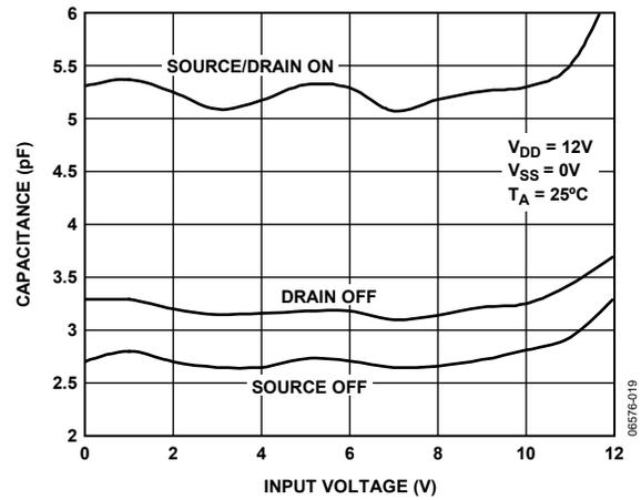
Figure 18. Capacitance vs. Input Voltage, Single Supply
