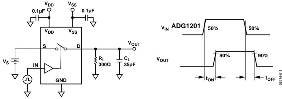
Figure 26. Switching Times
