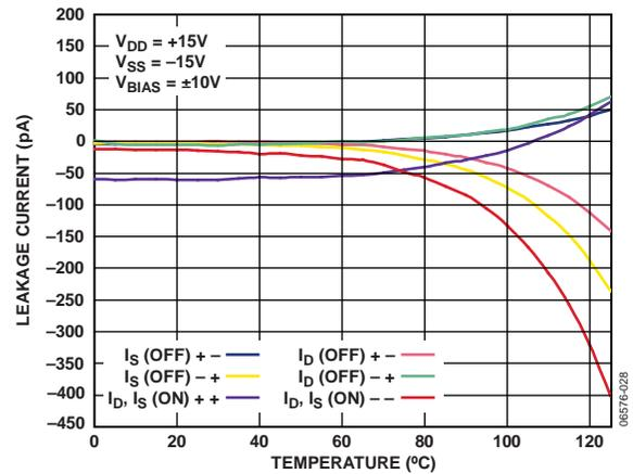
Figure 8. Leakage Current vs. Temperature, Dual Supply
