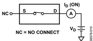
Figure 22. On Leakage
