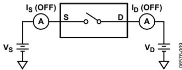
Figure 21. Off Leakage
