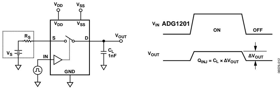
Figure 27. Charge Injection
