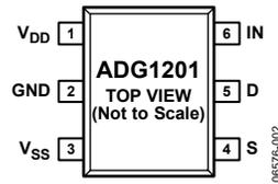
Figure 2. Pin Configuration
