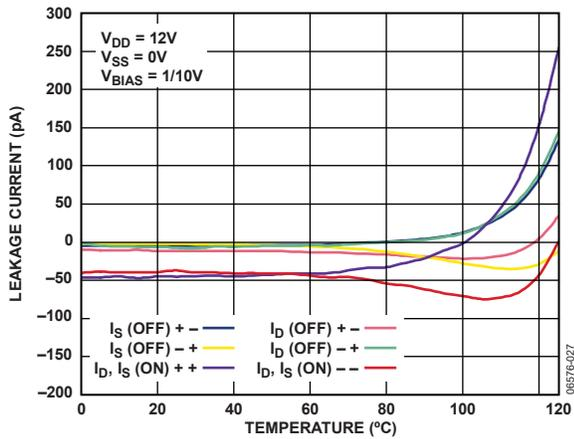
Figure 10. Leakage Currents vs. Temperature, Single Supply
