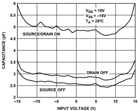
Figure 17. Capacitance vs. Input Voltage, Dual Supply
