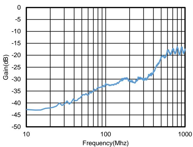
Figure 1. Off-Isolation, V<sub>CC</sub> = 5V
