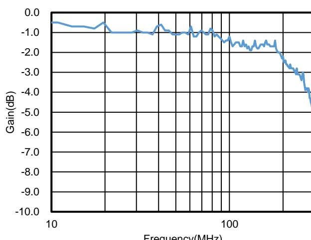
Figure 2. Bandwidth, V<sub>CC</sub> = 5V
