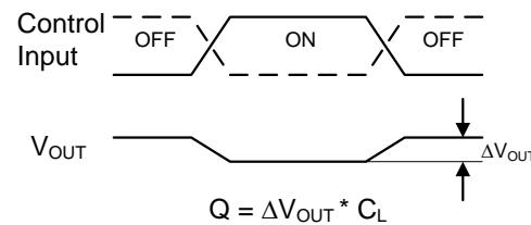
Figure 4 Charge Injection
