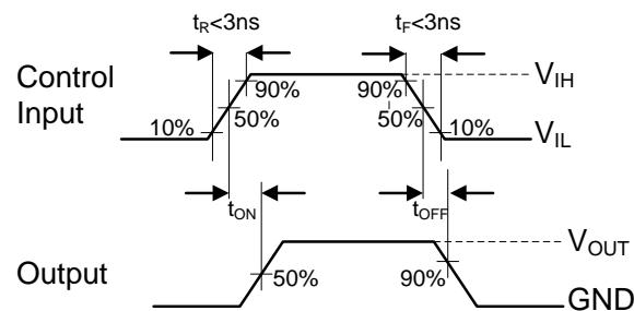
Figure 3 AC Test Circuit and Test Waveforms
