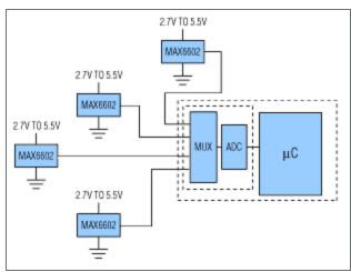
Figure 2. This simple approach to distributed temperature sensing is cost effective if the ADC resides on the  $\mu$ C and the mux has enough analog input channels to accommodate all sensors in the system.
