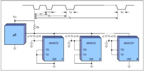
Figure 4. Using a time delay scheme to encode temperature information, the MAX6575 can transmit as many as eight temperatures to a single digital I/O pin at the  $\mu$ C.
