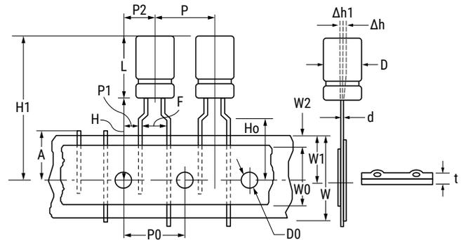
Fig. 3 (Diameter for  $\Phi 6$  to  $\Phi 8$ ) 6 – 8 mm EA
