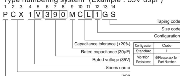
※ φ 6.3x8L(φ 6.3x8L), φ 8x10L(φ 8x10.5L), φ 10x10L(φ 10x10.5L), φ 10x12.7L(φ 10x13.2L) : The vibration structure-resistant product is also available upon request, please ask for details.
