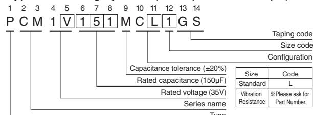
\* φ6.3x8L(φ6.3x8L), φ8x10L(φ8x10.5L), φ10x10L(φ10x10.5L), φ10x12.7L(φ10x13.2L) : The vibration structure-resistant product is also available upon request, please ask for details.
