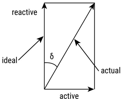
$\tan \delta$  is measured with the same set-up used for the series capacitance ESC.
