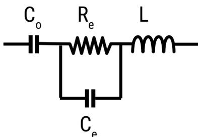
$C_o$  = Aluminum oxide capacitance (surface and thickness of the dielectric.)
