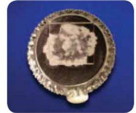
After 300 Cycles: Thermal grease voids and pumps out
