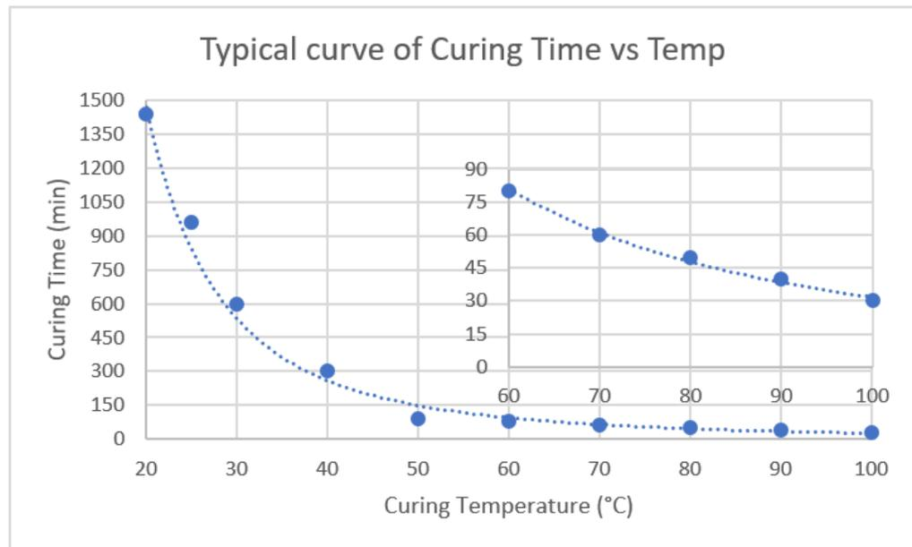
The above cure profiles are guideline recommendations. Cure conditions (time and temperature) may vary based on customers' experience and their application requirements, as well as customer curing equipment, oven loading and actual oven temperatures.
