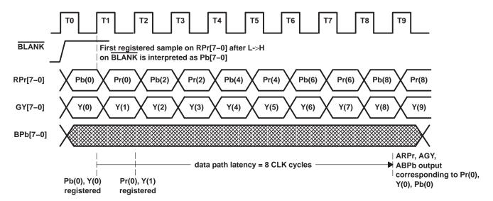
Figure 4. Input Format and Latency YPbPr 4:2:2 2×8 bit Mode
