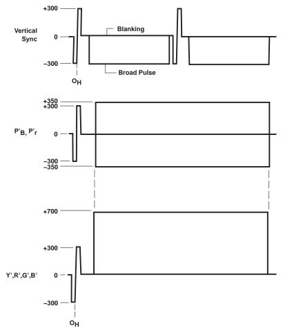
Figure 14. SMPTE 274M Analog Interface Horizontal Timing Details†
