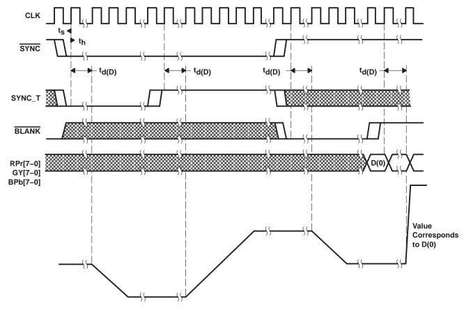
Figure 6. Sync and Blanking Generation
