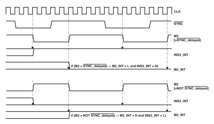
Figure 2. Generating INS3\_INT and M2\_INT from M2
