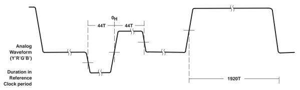
Figure 13. SMPTE 274M Line Waveform<sup>†</sup>
