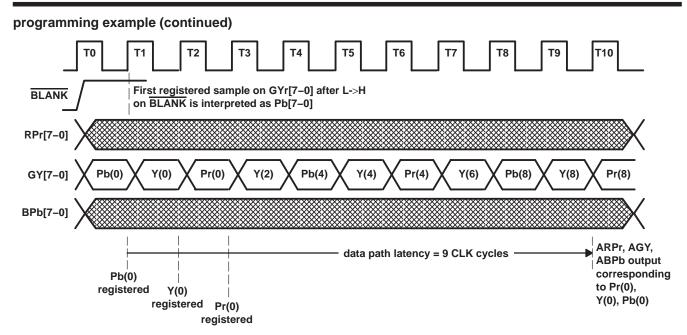
Figure 5. Input Format and Latency YPbPr 4:2:2 1×8 bit Mode
