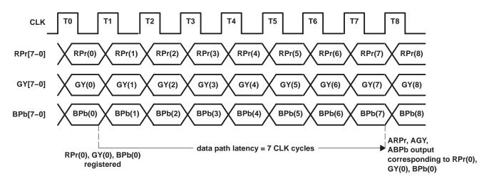
Figure 3. Input Format and Latency YPbPr 4:4:4 and GBR 4:4:4 Modes
