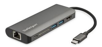
This USB-C multiport adapter with HDMI turns your MacBook Pro, Dell XPS, or other USB-C laptop into a workstation, anywhere you go. The USB Type-C multiport adapter provides 4K HDMI video output, a USB Type-C port (data/power), two USB 3.0 Type-A ports, a Gigabit Ethernet port and an SD card reader slot, all through one connection to your laptop's USB-C or Thunderbolt 3 port. Plus, it offers advanced charging through USB Power Delivery 3.0.
