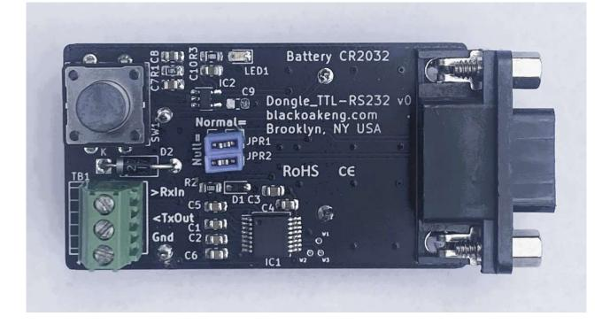
*Description.* Many electronic devices expose the UART only as logic (TTL) levels. In order to interface with a traditional RS232 port, the signals must be converted to higher, bipolar voltages. That's what the Dongle does. It is self-powered; it does not need a separate power source. It has digital input and output lines on a terminal block, so any device can be wired in. It also has shunts to change the Dongle from Normal operation to Null modem. The RS232 connector is a standard DSub-9.
