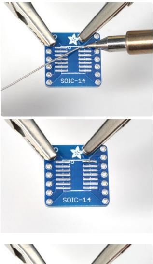
We'll start by melting a little solder on one corner pad. I like going with the top right corner. Melt just a tiny bit on, so its rounded but not blobby
