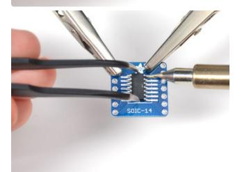
Once you've identified which is pin 1, hold the chip with the tweezers over the pads and then re-heat the corner pad you soldered onto a few steps ago.
