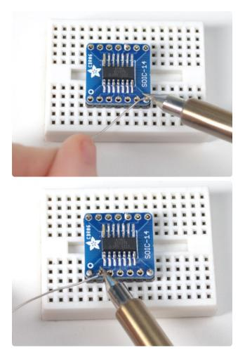
Almost done, now all you have to do is solder each header pin into the corresponding hole to make a secure connection
