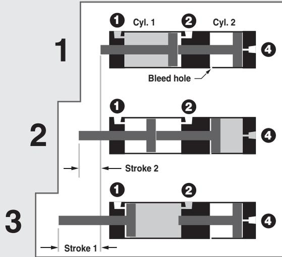
Exposed rod is in retracted "home" position when port 1 is pressurized and ports 2 & 4 are open to atmosphere.
