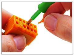
Covering unused clamping units in CAGE CLAMP®-equipped male and female connectors (e.g., when doubling the pin spacing to meet clearance and creepage distance requirements, or when a higher rated voltage is required). Lockout pins are not suitable for panel-mount, angled female connectors.
