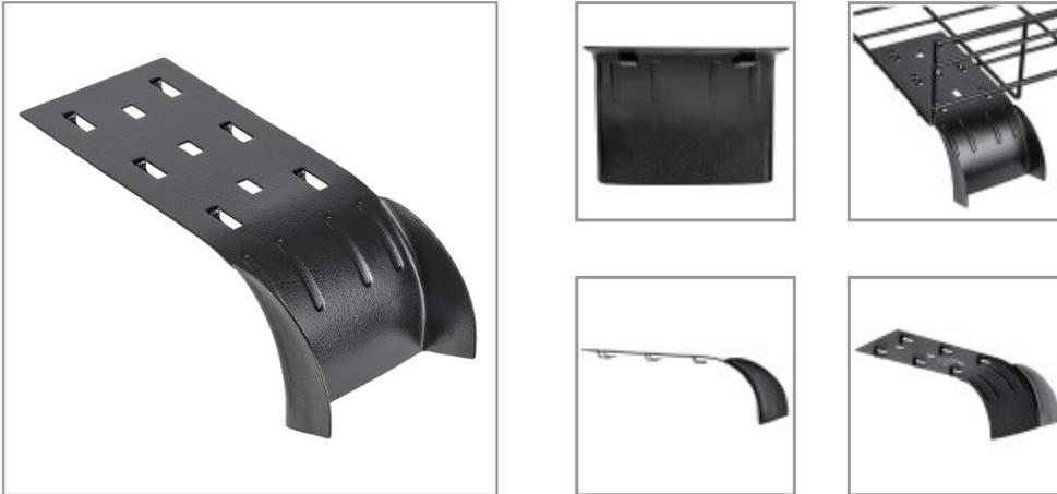
Metal cable dropout maintains a proper bend radius for copper cables that are routed down the side of your wire mesh cable tray.
