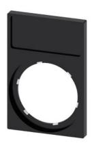
Label holder, frame rectangular at the bottom, black, for labeling plate 12.5 mm x 27 mm for gluing, Z=100-unit packaging
