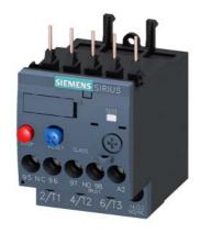
Overload relay 3.5...5.0 A Thermal For motor protection Size S00, Class 10 Contactor mounting Main circuit: Screw Auxiliary circuit: Screw Manual-Automatic-Reset Multi-unit packaging Pack = 16 units
