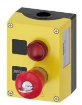
Enclosure for command devices 22 mm, round, enclosure material plastic, enclosure top part yellow, 2 control points plastic, B = Indicator light, red, LED 24 V AC/DC,screw terminal, label without inscription, A = EMERGENCY STOP, 40 mm, RONIS SB30, label with inscription: EMERGENCY STOP, 1 NO, 1 NC, screw terminal, floor mounting, 1xM20 each on top and bottom labels enclosed
